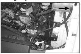
15b. Install the supplied coolant recovery hose and secure with the provided hose clamps.
