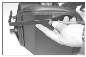
15. Install the provided "L" bracket onto the heat shield using the provided hardware as shown.
