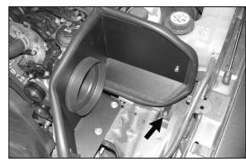
16. Install the heat shield into the vehicle and secure the "L" bracket to the threaded hole on the inner fender using the provided hardware as shown but do not tighten at this time.
