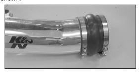
19. Install the silicone hose and hose clamps onto the K&N® intake tube as shown.
