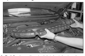
3. Pull firmly on the stock intake tube to release it from the stock air cleaner and the inner fender, then, remove the stock intake tube as shown.
