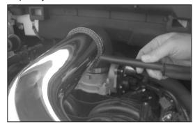
17a. On vehicles equipped with the brake booster vent line install the K&N® intake tube into the silicone hose at the throttle body. Align the brake booster vent line to the K&N® intake tube as shown and place a mark for drilling location.
