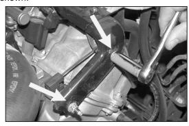
10. On vehicles equipped with the intake tube support bracket, reinstall the two nuts removed in step nine as shown.
