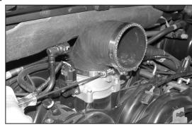
17. Install the  $90^{\circ}$  silicone hose and hose clamps onto the throttle body as shown but do not tighten completely at this time.
