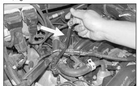
22. Remove the stock crankcase vent hard line as shown.
