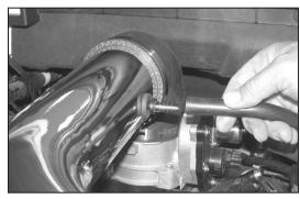
23a. On vehicles equipped with brake booster vent lineInstall the provided hose mender into the grommet in the intake tube and connect the brake booster vent line to the hose mender.
