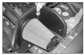
24. Install the K&N® air filter and tighten the provided hose clamp as shown.
