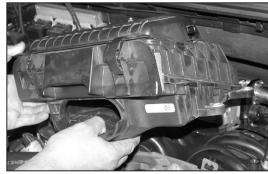
8. Pull firmly upwards to remove the air cleaner as
