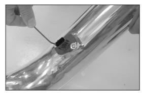
18. Install the mass air sensor into the K&N<sup>®</sup> Intake tube and secure with the provided hardware as shown.
