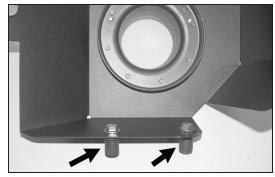
13. Install the provided rubber inserts, hex bolts and washers onto the heat shield as shown, but do not tighten at this time.
