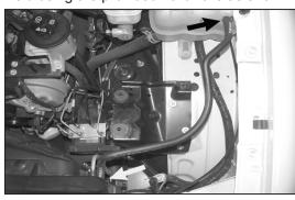
15a. Loosen the coolant recovery hose, hose clamps, and then remove the factory recovery hose shown. Be sure to catch any coolant, which flows out of the radiator during hose removal.
