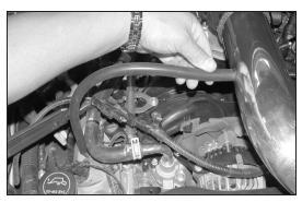
23. Install the provided silicone hose onto the vent on the cam cover, then, connect the other end to the vent on the K&N® intake tube as shown.
