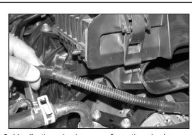
6. Unclip the wire harness from the air cleaner as shown.
