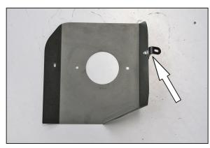
7. Install the heat shield mounting bracket (064323) onto the heat shield as shown using the provided hardware.
