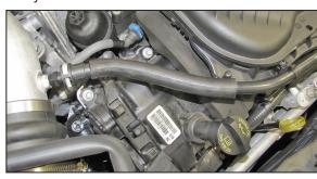
20. Install the factory quick disconnect fitting into the provided crank case vent hose and then install the assembly onto the factory hardline and connect the quick disconnect fitting to the fitting installed into the K&N® intake tube.
