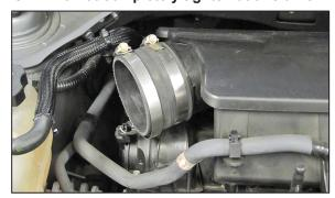
14. Install the provided coupler hose (08690) onto the intake plenum and secure with the provided hose clamp.
