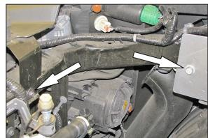
Remove the two factory bolts shown.
