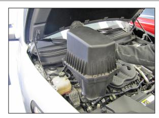
5. Lift up the air filter housing to dislodge it from the mounting grommets and then remove the complete air filter housing assembly from the vehicle.
