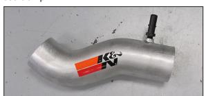
15. Install the provided quick disconnect fitting into the  $K\&N^{\otimes}$  intake tube as shown.
