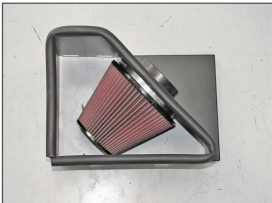
9. Install the K&N® air filter onto the filter adapter and secure with the provided hose clamp.
