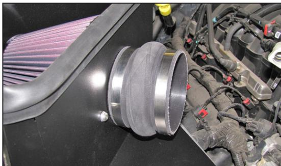
15. Install the provided coupler hump hose (08418) onto filter adapter and secure with the provided hose clamp.
