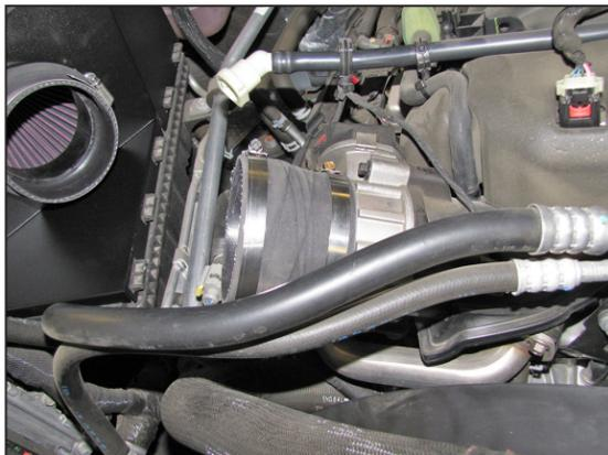
16. Install the provided step coupler (08497) onto the throttle body and secure with the provided hose clamps.
