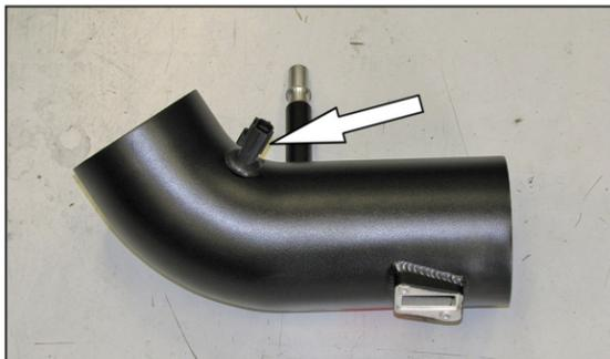
13. Remove the O-ring from the inlet air temperature sensor and then install the sensor into the grommet installed into the K&N® intake tube during the previous step.
