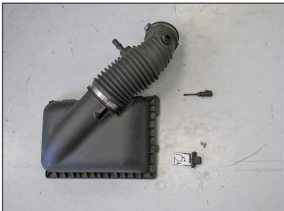
11. Remove the two screws securing the humidity sensor then remove the humidity sensor from the air filter housing. Remove the inlet air temperature sensor from the stock intake tube.
