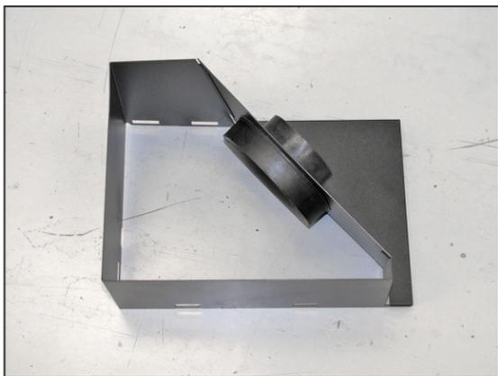
7. Install the filter adapter into the K&N® heat shield as shown and secure with the provided hardware.
