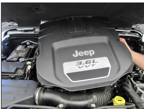
2. Lift up and remove the engine cover.
