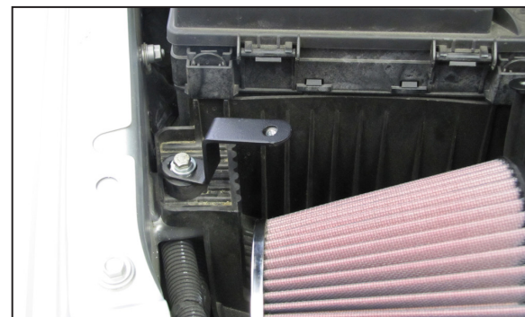
21. Install the provided bracket (083163) onto the rubber mounted stud using the provided hardware.
