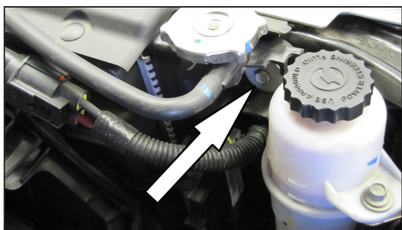
10. Remove the bolt shown that secures the radiator to the core support.
