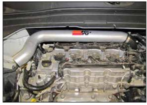
17. Install the K&N<sup>®</sup> intake tube assembly into the coupling hose and align the bracket with the mounting lug on the valve cover. Tighten the hose clamps but do not secure the bracket to the valve cover.
