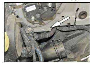
that are not equipped with a humidity sensor, install the provided gasket onto the block off and then install the block off into the K&N<sup>®</sup> intake tube and secure with the provided hardware.
