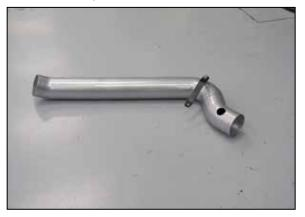
11. Install the tube mounting bracket (064335) onto the K&N $^{\odot}$  intake tube as shown using the provided hardware.
