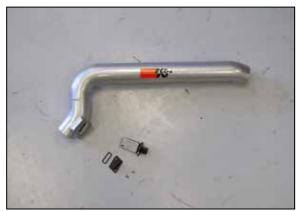
10. On vehicles equipped with a mass air sensor, install the sensor into the  $K\&N^{\otimes}$  intake tube and secure with the provided hardware. On vehicles
