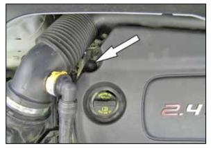
2. Remove the bolt securing the engine cover and then remove the engine cover from the vehicle. NOTE: This bolt will be reused in a later step.
