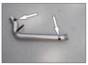
12. Install the two provided grommets into the  $K\&N^{\otimes}$  intake tube as shown.
