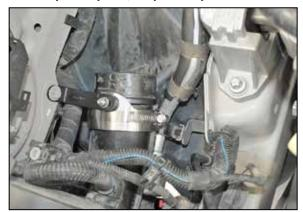
23. Install the saddle assembly onto the inner fender using the factory bolt removed in step #18 and then secure the fresh air intake duct with the provided hose clamp.
