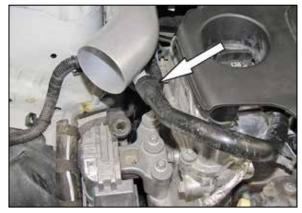
20. Connect the crank case vent hose to the fitting installed into the K&N<sup>®</sup> intake tube. **NOTE: Connect mass air sensor if equipped.**
