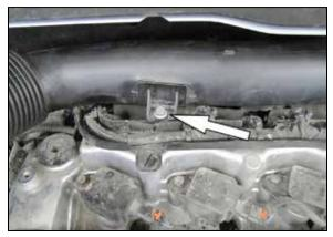
4. Remove the bolt that secures the intake tube to the valve cover.
