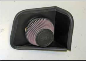
27. Install the K&N<sup>®</sup> air filter onto the filter adapter and secure with the provided hose clamp.
