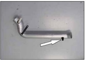
15. Remove the O-Ring from the sensor and then install the sensor into the grommet installed into the  $K\&N^{\mbox{\ensuremath{\$}}}$  intake tube.
