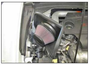
28. Install the filter assembly onto the K&N<sup>®</sup> intake tube and adjust for best fit and then secure with the provided hose clamp.
