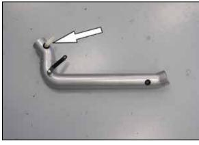
13. Install the 90° vent fitting into the grommet installed into the K&N $^{\circ}$  intake tube as shown.
