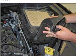
9. Lift up the lower air box to dislodge it from the mounting grommets and then remove the lower air box from the vehicle. Some vehicles may have a power steering line attached to the airbox that will need to be unhooked.
