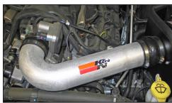
21. Install the K&N® intake tube into the hump hose at the filter adapter and then into the hose at the throttle body. Adjust the tube and heat shield for best fit and clearance and then secure with the provided hose clamps
