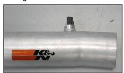
19. Install the inlet air temperature sensor into the K&N® intake tube.
