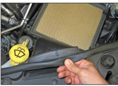
8. Unhook the sealing trim from the fresh air intake scoop.
