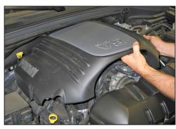
2. Lift up the engine cover to dislodge it from the mounting grommets and remove it from the vehicle.
