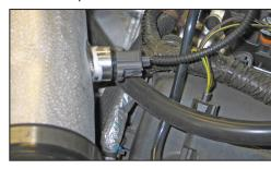
23. Connect the inlet air temperature sensor extension harness into the factory electrical connection and then connect the other end into the inlet air temperature sensor as shown.
