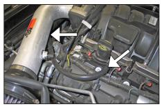
22. Install the crank case vent hose onto the 90° vent fitting and then attach the open end to the valve cover port.
