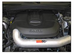
27. Adjust the intake kit for proper fit and then secure the mounting hardware and hose clamps. Reinstall the factory engine cover.
