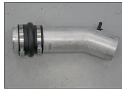
22. Slide the provided silicone hump hose (5-576) all the way onto the K&N $^{\circ}$  intake tube #27446 as shown.
