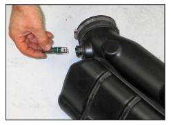
17. Remove the inlet air temperature sensor from the factory intake tube.
