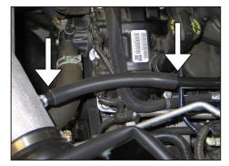
26. Install the provided crank case vent hose onto the vent fitting attached to the K&N<sup>®</sup> intake tube. Connect the open end of the crank case vent tube to the factory crank case vent tube that was cut in the previous step.
