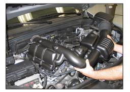
6. Remove the intake tube and upper air box from the vehicle as shown.
