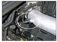
24. Reconnect the inlet air temperature sensor electrical connection.
