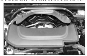
3. Remove the oil filler cap and then lift up the front of engine cover to gain access to the intake plenum hose clamp at the throttle body and plenum mounting bolt.
