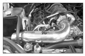
29. Install the K&N® intake tube into the silicone hose at the throttle body and onto the tube mounting bracket, then secure with the provided hose clamp and hardware.
