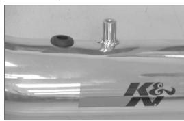
25. Install the provided grommet into the K&N® intake tube as shown.
