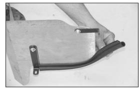
18. Install the sort edge trim onto the heat shield assembly as shown.
