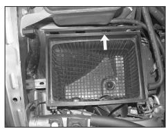
13. Remove the air box mounting bolt shown.
