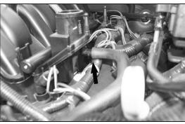
8. Remove the crank case vent hose from the valve cover.
