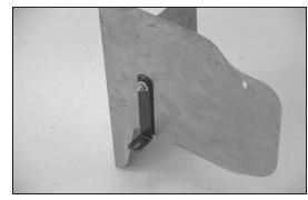
16. Install the long "L" bracket (26626) onto the heat shield as shown with the provided hardware.
