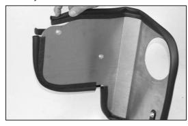
19. Install the long edge trim onto the heat shield as shown.
