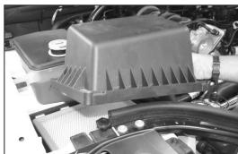
9. Unhook the air box lid retaining clamps and then remove air box lid and filter.
