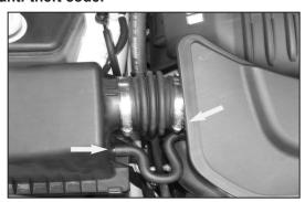
2. Loosen the hose clamp, which secures the stock intake tube to the intake plenum, and disconnect the crank case vent hose from the air box lid.
