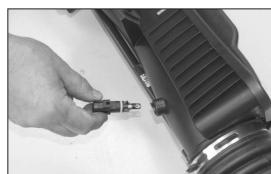
26. Rotate the air temperature sensor counter clockwise and remove the sensor from the stock intake plenum as shown.
