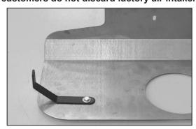
15. Install the supplied "C" bracket (07171) onto the heat shield as shown with the provided hardware. NOTE: Due to manufacturing tolerances, it may be necessary to us the provided spacer and longer bolt to attach the mounting bracket to the heat shield. This will enable the mounting bracket to align with the longer air box mounting brackets on some vehicles.
