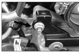
23. Remove the intake plenum mount nut shown. **NOTE: Do not discard as this nut will be reused.**
