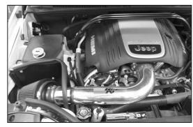
36. Reinstall the engine cover and oil filler cap. Reconnect the vehicle's negative battery cable. Double check to make sure everything is tight and properly positioned before starting the vehicle.
