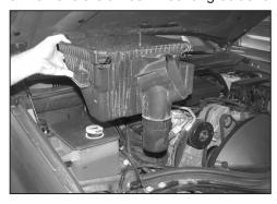
14. Lift the lower air box and remove it from the vehicle as shown.
