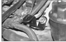
23. Install the tube mounting bracket onto the A/C compressor and secure with the factory mounting bolt removed in step #22.
