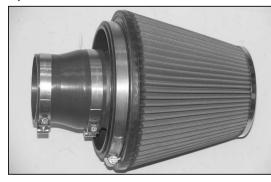
33. Install the silicone hose (084055) onto the air filter assembly and secure with the provided hose clamp.
