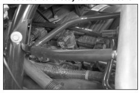
30.Install the supplied silicone hose onto the crankcase vent "T" and connect the other end onto the K&N® intake tube as shown.
