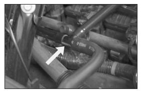
29. Remove the factory crankcase vent hose from the "T" fitting shown.
