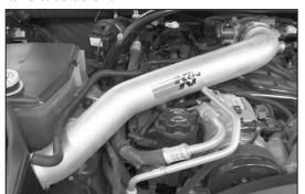
28. Install the K&N®intake tube into the silicone hose at the throttle body and align with the tube mounting bracket installed in step #23. Secure with the provided hardware and hose clamp.
