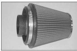
32. Install the filter adapter into the air filter as shown, secure with the provided hose clamp.
