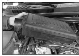
20c. Remove the intake plenum from the vehicle as shown.
