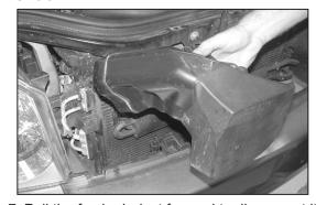
7. Pull the fresh air duct forward to disconnect it from the airbox and then remove it from the vehicle.
