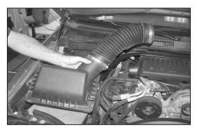
3. Unclip the upper airbox retaining clips and remove the upper airbox and intake tube assembly as shown.
