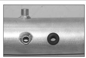
25. Install the supplied rubber grommet into the K&N® intake tube as shown.
