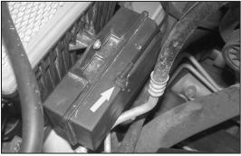
4. Disconnect the vacuum canister hose shown. NOTE: Some vehicles may not be equipped with a vacuum canister.
