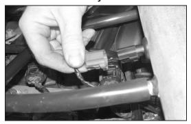
31. Connect the air temperature sensor electrical connection.
