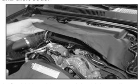
2. On 2008 and later model vehicles, pull up on the engine cover to dislodge it from the mounting grommets and then remove the engine cover from the vehicle.
