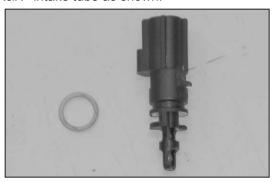
26. Remove the rubber sealing "O" ring from the air temperature sensor as shown.
