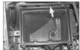
8. Remove the airbox mounting bolt shown.
