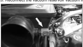
20a. Disconnect the air temperature electrical connection.
