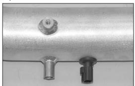
27. Install the air temperature sensor into the K&N<sup>®</sup> intake tube as shown.
