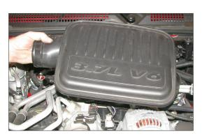
5. Lift to dislodge the intake plenum from it's mounting grommets and remove the intake plenum from the vehicle as shown.
