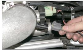
22. Reconnect the air temperature sensor electrical connection as shown.
