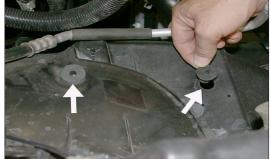
12. Install the two threaded inserts into the air box mounting grommet locations as shown.
