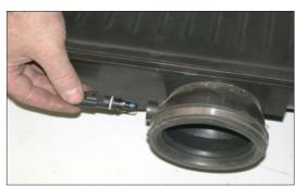
17. Twist the air temperature sensor counter clockwise and remove it from the stock intake plenum.
