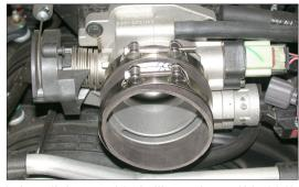
16. Install the provided silicone hose (084031) onto the throttle body and secure with the provided hose clamp as shown.
