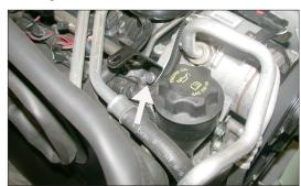
15. Install the tube mounting bracket (010119) onto the A/C compressor using the bolt removed in step #14 as shown.
