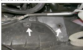
6. Pull the two-air box mounting grommets shown from the inner fender.
