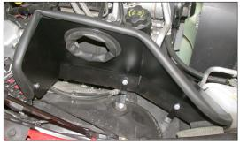
13. Install the heat shield assembly and secure with the provided hardware and the factory air box mounting nut.
