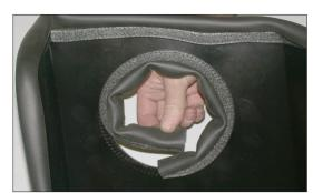
11. Install the provided edge trim onto the heat shield as shown.
