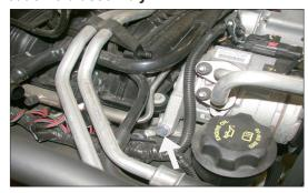
14. Remove the rear, lower A/C compressor mounting bolt shown.
