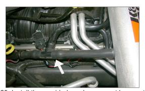
23. Install the provided crank case vent hose onto the factory "TEE" fitting and then onto the K&N<sup>®</sup> intake tube as shown.
