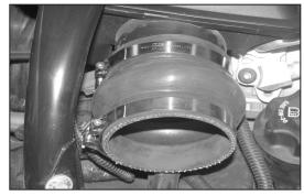
23. Install the silicone hose (084056) onto the intake plenum and secure with the provided hose clamp as shown.
