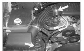
2. Loosen the hose clamp, which secures the stock
