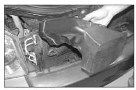
7. Pull the fresh air duct to disconnect it from the airbox and then remove it from the vehicle.
