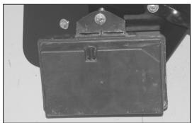
17.On vehicles equipped with vacuum reservoir, using the provided spacer, install the vacuum reservoir onto the heat shield as shown. **NOTE: Due to manufacturing tolerances, 2 spacers may be needed.**
