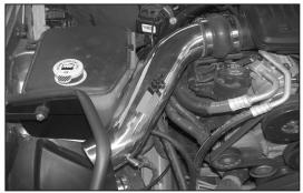
24. Install the K&N<sup>®</sup> intake tube into the silicone hose at the throttle body and onto the bracket. Secure the tube with the provided hose clamp and hardware.
