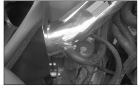
25. Connect the crankcase vent hose onto the K&N<sup>®</sup> intake tube as shown and secure with the provided hose clamp.
