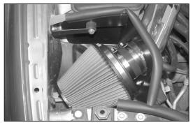
28. Install the air filter assembly onto the K&N<sup>®</sup> intake tube as shown and secure with the provided hose clamp.
