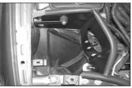
21. Install the heat shield assembly into the vehicle and secure it to the mounting locations with the provided hardware. 26. Install the filter adapter into the air filter as shown, secure with the provided hose clamp.
