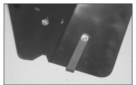
12. Install the "L" bracket (070952) onto the heat shield with provided hardware as shown. NOTE: The bracket mounts on the inside of the heat shield with the "L" positioned to the outside of the heat shield.
