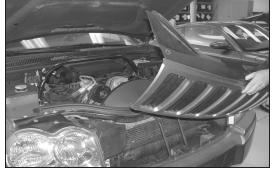
6. Remove the six grill retaining clips from the grill, then tilt the grill froward and remove from the vehicle.
