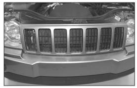
29. Reinstall the grill assembly with the factory retaining clips removed in step #5.
