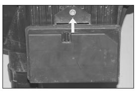
16. On vehicles equipped remove the bolt which secures the vacuum reservoir to the airbox and then remove the reservoir from the airbox.
