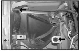
18. Remove the coolant reservoir retaining nut and airbox mounting grommet shown.
