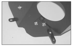
15. Install the twist bracket onto the heat shield as shown using the provided hardware.
