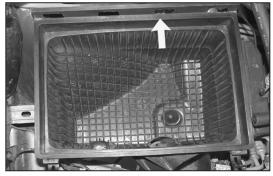
8. Remove the airbox mounting bolt shown.
