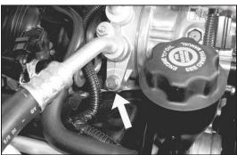
21. Remove the A/C compressor-mounting bolt.
