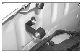
13. On vehicles that did not come with a TCM, mount "L" bracket onto existing stud with the provided hardware.
