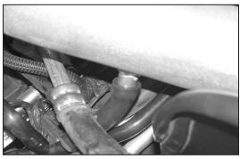
36. Connect the supplied crank case vent hose onto the  $K\&N^{\mbox{\scriptsize @}}$  intake tube.
