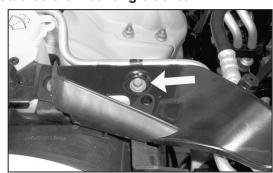
14. Remove the 6mm bolt from core support.
