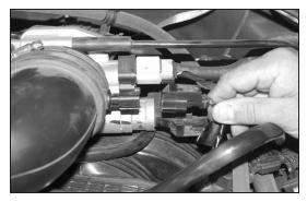
4. On vehicles equipped with an intake air temperature sensor, disconnect the electrical connection from the air temperature sensor as shown
