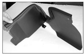
17. Install edge trim onto heat shield as shown. NOTE: Some trimming of the edge trim will be necessary.
