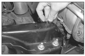
19. Vehicles that do not come equipped with cruise control, install the provided spacer and washer onto the stud as shown.
