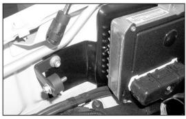
12. Secure "L" bracket to inner fender with the nut that was removed in the previous step.
