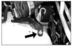
18. Install the provided ¼ washer onto existing nut that retains the cruise control bracket to vehicle.
