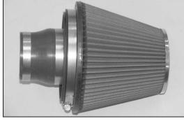
38. Install the silicone (084055) onto the filter adapter and secure with the provided hose clamp.
