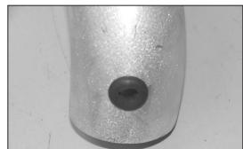
27. Install the supplied rubber grommet into the hole drilled into the K&N $^{\! \odot}$  intake tube as shown.
