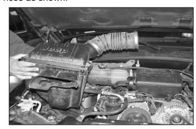
3. Firmly lift up to disengage the air box from the mounting grommets and remove the air box from the vehicle.
