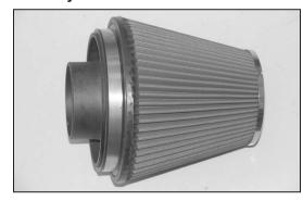
37. Install the filter adapter into the air filter as shown and secure with provided hose clamp.
