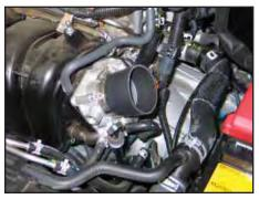
13. Install the provided silicone hose (084016) onto the throttle body and secure with the provided hose clamp.
