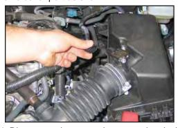
4. Disconnect the mass air sensor electrical connection. Then unhook the mass air sensor wiring harness from the upper air box.
