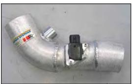
15. Install the mass air sensor into the K&N<sup>®</sup> intake tube and secure with the provided hardware.
