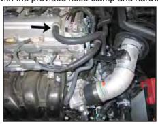
21. Install the crank case vent hose onto the valve cover port and then onto the vent chamber installed into the K&N® intake tube.
