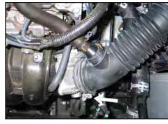
5. Loosen the hose clamp which secures the intake tube to the throttle body.
