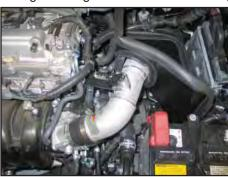
20. Install the K&N® intake tube into the silicone hose at the throttle body and align with the bracket installed in the previous step. Secure the intake tube with the provided hose clamp and hardware.
