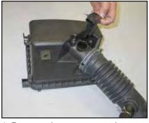
14. Remove the two screws that secure the mass air sensor to the upper air box and then remove the mass air sensor as shown.
