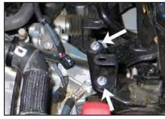
9. Install the two heat shield mounting brackets (070052) onto the air box mounting bracket as shown
