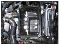
7. Remove the three lower air box retaining bolts. Then unclip the wiring harness from the rear of the air box and remove the lower air box housing from the vehicle.
