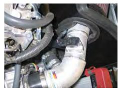
21a. Route the mass air electrical harness through the heat shield as shown and then reconnect the mass air sensor electrical connection.
