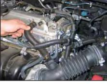
3. Disconnect the crank case vent hose from the valve cover port as shown.
