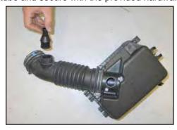
16. Remove the crank case vent chamber from the stock intake tube.
