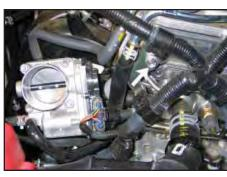
8. Remove the bolt shown which secures the engine wiring harness to the engine.
