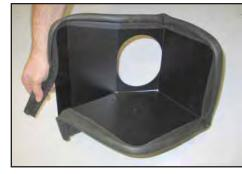
10. Install the provided long edge trim onto the heat shield as shown.
