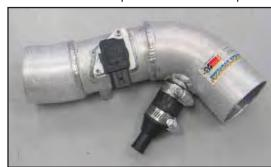
18. Install the vent crank case vent chamber into the silicone hose and secure with the provided hose clamp.
