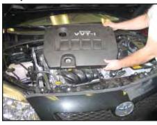
2. Pull up firmly to dislodge the engine cover from the mounting grommets and then remove the cover from the engine.
