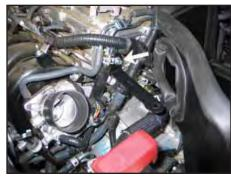
19. Install the tube mounting bracket (070110) onto the engine using the bolt removed during step #8.
