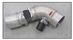
17. Install the silicone hose onto the K&N<sup>®</sup> intake tube and secure the provided hose clamp.
