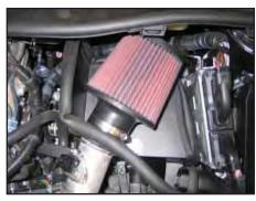
22. Install the K&N® air filter onto the intake tube and secure with the provided hose clamp.
