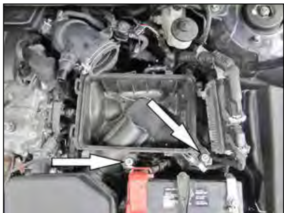
7. Remove the two bolts securing the lower air box to the vehicle, then pull the lower air box up to release it from the mounting grommet, disconnect it from the fresh air intake duct and remove it from the vehicle.
