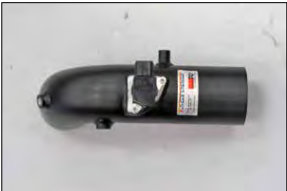
20. Install the mass air sensor into the K&N® intake tube and secure with the provided hardware.
