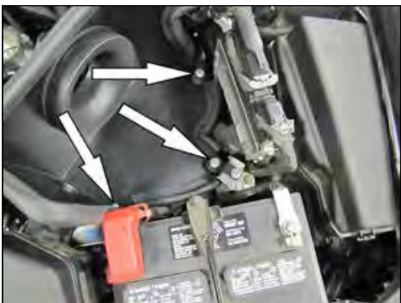
17. Install the heat shield into the vehicle so the fresh air duct slides over the tube on the heat shield and the heat shield sits on the mounting locations. Secure the heat shield to the rubber mounted studs and brackets with the provided hardware. NOTE: Use "Z" bracket (070061) at the center mounting location.
