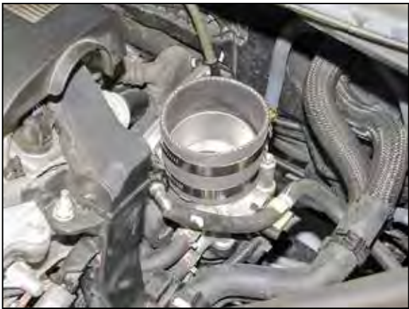
18. Install the provided silicon hose (08434) onto the throttle body and secure with the provided hose clamp.
