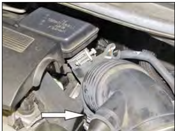
9. Loosen the hose clamp securing the intake hose to the throttle body and remove the intake hose from the vehicle. NOTE: K&N Engineering, Inc., recommends that customers do not discard factory air intake.
