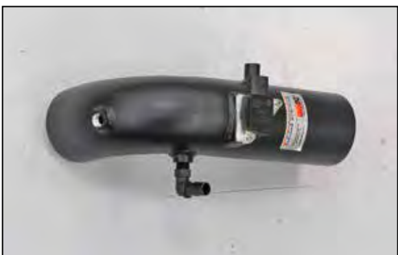
21. Install the 90° vent fitting into the K&N® intake tube as shown. NOTE: Plastic NPT fittings are easy to cross thread. Install the vent fitting "hand" tight, then turn it two complete turns with a wrench.
