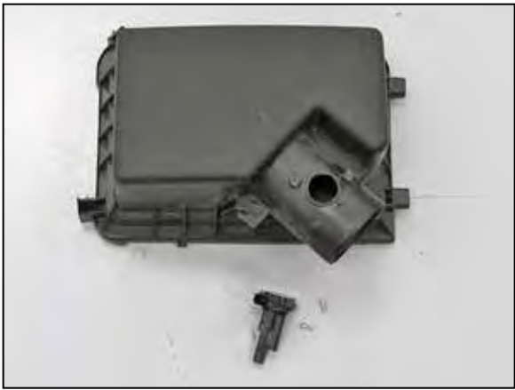
19. Remove the two screws securing the mass air sensor into the upper air box and then remove the mass air sensor from the upper air box.
