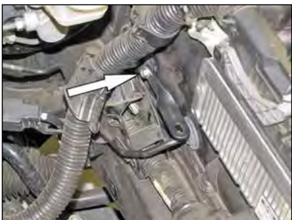
15. Install the heat shield mounting bracket (070702) onto the inner fender air box mounting location from step #10.
