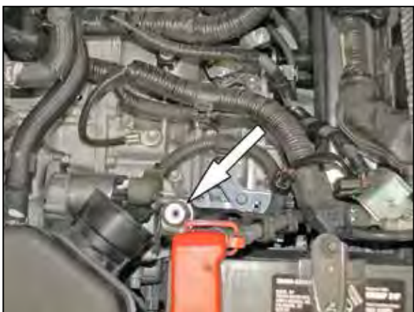
16. Install the 1" rubber mounted stud onto the front air box mounting location as shown.
