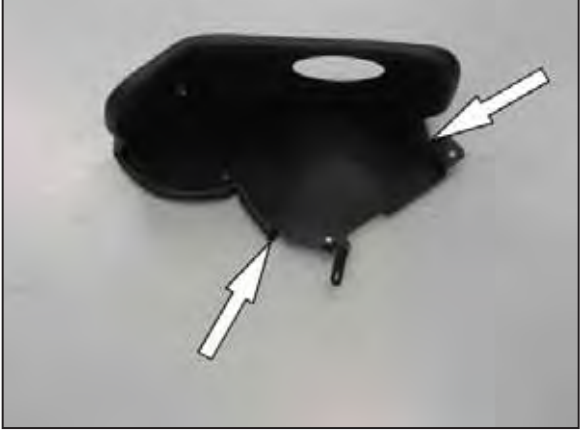
20. Install the 47" long section of edge trim onto the heat shield as shown.
