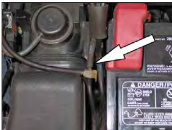
8. Disconnect the vacuum line at the TEE fitting shown.
