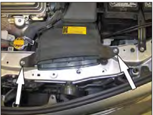
13. Remove the two bolts securing the fresh air duct and then remove the fresh air duct from the vehicle.
