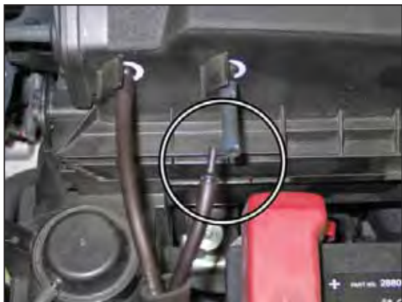
7. Disconnect the vacuum line from the union fitting shown leaving the union installed into the vacuum line attached to the vehicle.
