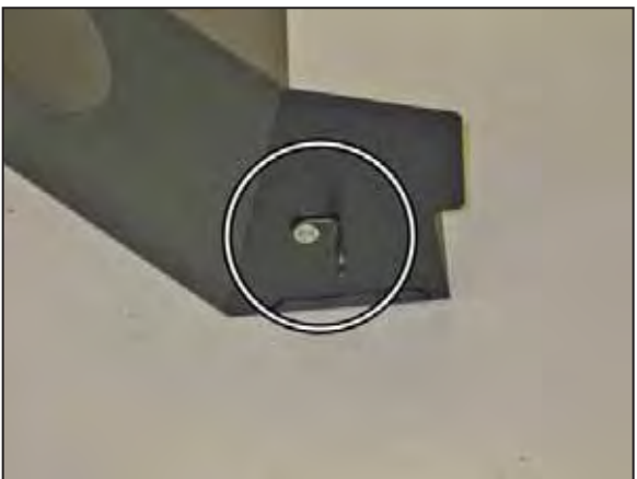
17. Install the heat shield mounting bracket (070066) onto the heat shield using the provided hardware. NOTE: The slotted end of the bracket attaches to the heat shield.
