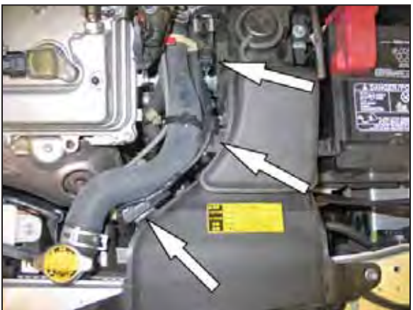
12. Disconnect the vacuum switch electrical connection and then unhook the harness from the fresh air duct.
