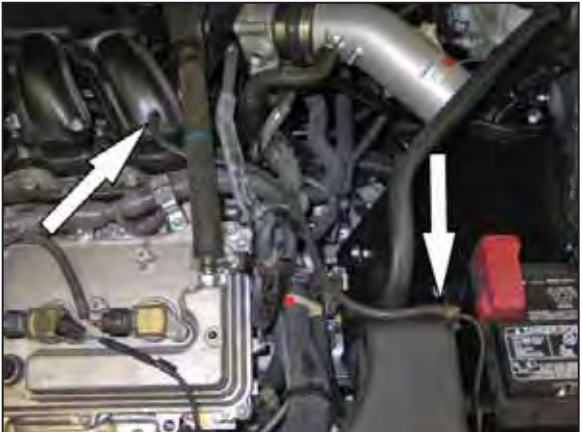
36. Install the provided longer vacuum hose to the vacuum TEE and install the open end onto the intake plenum.
