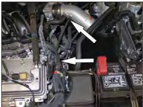
37. Connect the shorter provided vacuum line to the open factory union fitting and then connect the open end to the K&N® intake tube.
