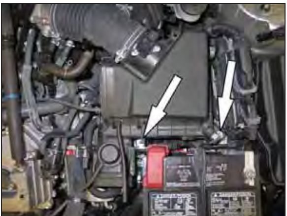
14. Remove the two bolts shown securing the air box.
