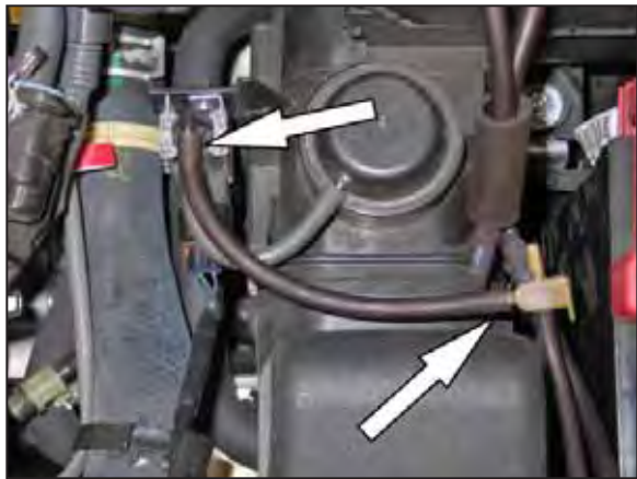
9. Remove the vacuum hose shown from the TEE fitting and vacuum switching valve.
