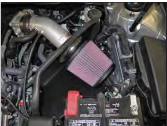
41. Install the K&N® air filter and secure with the provided hose clamp.
