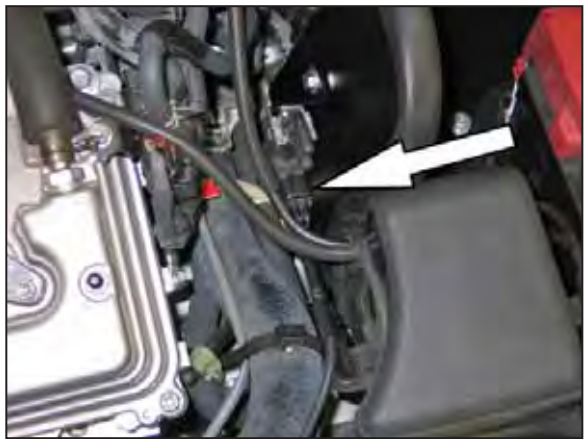
38. Reconnect the vacuum switching valve electrical connection and secure the wiring harness to the fresh air intake scoop.
