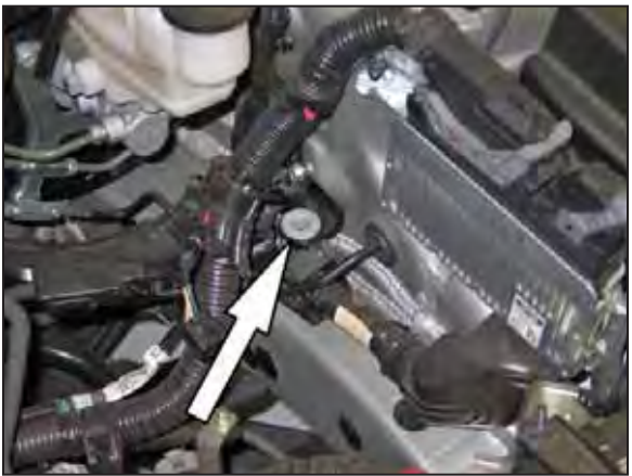
16. Remove the air box mounting grommet shown.
