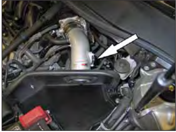
40. Reconnect the mass air sensor electrical connection.
