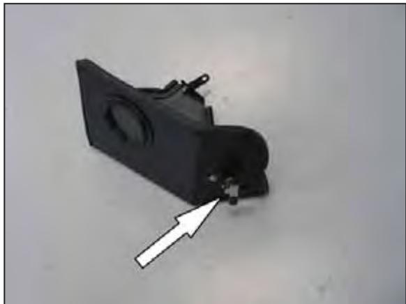
24. Secure the vacuum switching valve to the "L" installed onto the heat shield as shown and then install the provided vacuum caps.
