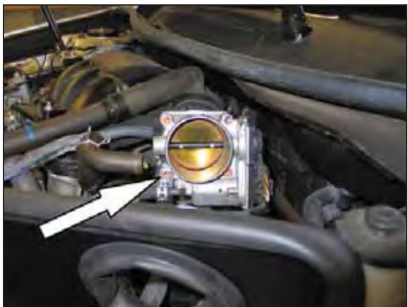
27. Remove the front lower throttle body mounting bolt shown. NOTE: This bolt will be reused in the next step.
