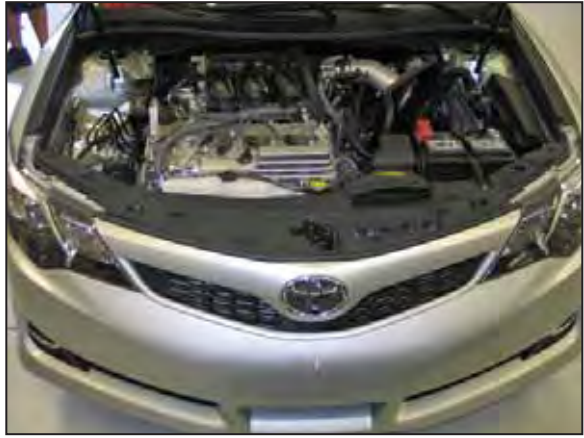
39. Reinstall the valence and secure with the factory retaining clips.
