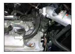
26. Attach the provided crank case vent hose to the 90° vent fitting in the K&N<sup>®</sup> intake tube and to the valve cover port as shown.
