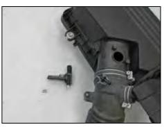
21. Remove the mass air sensor from the factory upper air box.
