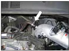
25. On vehicles equiped with EVAP valve, attach the EVAP vent line to the straight fitting installed in the K&N® intake tube.
