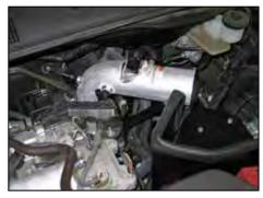
23. Install the K&N® intake tube into the silicone hose at the throttle body and align with the mounting bracket previously installed. Secure the tube with the provided hose clamp and hardware.
