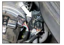
6. Lift up and remove the EVAP solenoid from the rear of the factory intake tube.
