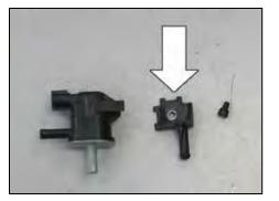
15. On vehicles equiped with EVAP valve, remove the EVAP control valve mounting bracket from the EVAP control valve.
