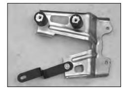
13. Install the heat shield mounting bracket (26655) onto the air box mounting bracket as shown. NOTE: The long leg of the bracket is attached to the bracket.
