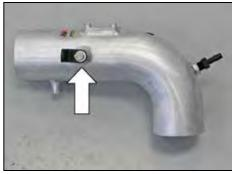
20. On vehicles equiped with EVAP valve, install the provided EVAP mounting bracket (070066) onto the K&N® intake tube using the provided hardware.
