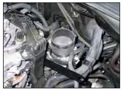
17. Install the provided silicone hose (08192) onto the throttle body and secure with the provided hose clamp.
