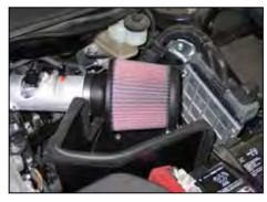
27. Install the K&N<sup>®</sup> air filter onto the intake tube and secure with the provided hose clamp. NOTE: Drycharger<sup>®</sup> air filter wrap; part # RX-4990DK is available to purchase separately. To learn more about Drycharger<sup>®</sup> filter wraps or look up color availability please visit http://www.knfilters.com<sup>®</sup>.
