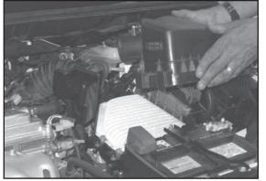
5. Loosen the hose clamp that secures the intake tube to the upper air box. Then, un-hook the three upper air box retaining clips. Remove the upper air box from the vehicle as shown.
