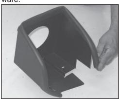
14. Install the long edge trim onto the heat shield as shown.
