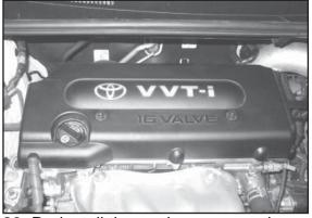
23. Re-install the engine cover and secure with the factory nuts.
