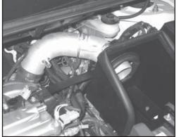
19. Install the K&N intake tube into the silicone hose at the throttle body and align with the mounting bracket. Secure the EVAP bracket and mounting bracket in the same location on the intake tube using the provided hardware.
