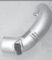
18. Install the mass air sensor into the K&N intake tube and secure with the provided hardware as shown.
