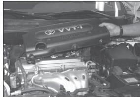
2. Remove the two nuts that secure the engine cover, then remove the engine cover from the engine as shown.
