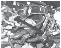
11. Install the tube mounting bracket (#06509) onto the cylinder head using the bolt removed in the previous step.
