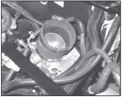
12. Install silicone step hose (#08713) onto the throttle body and secure with the provided hose clamp.
