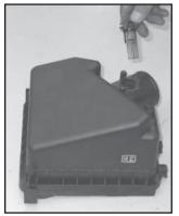
17. Remove the two screws that secure the mass air sensor to the stock air box. Then, remove the mass air sensor as shown.
