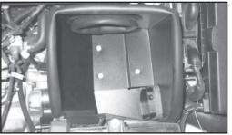
16. Install the heat shield assembly and secure with the provided hardware.Note: The fresh air supply tube is to be installed into the heat shield.
