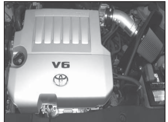
35. Reconnect the vehicle's negative battery cable. Check to ensure all hose clamps and fittings are properly tightened and positioned correctly before starting the vehicle.
