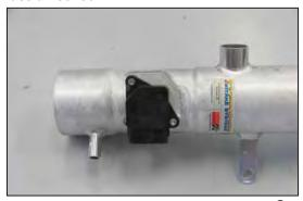
16. Install the mass air sensor into the  $K\&N^{\textcircled{8}}$  intake tube and secure with provided hardware.
