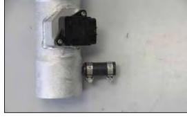
19. Install the newly cut 1-3/4" long silicone hose (08415) onto the  $K\&N^{\circledR}$  intake tube and secure with the provided hose clamp as shown in the photograph.
