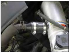
22. Install the crank case vent hose/chamber into the silicone hose installed onto the K&N<sup>®</sup> intake tube in step 19; secure with the provided hose clamp.
