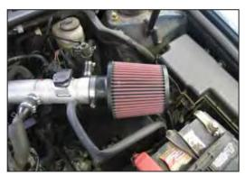
25. Install the  $K\&N^{\circledR}$  air filter onto the intake tube; secure with the provided hose clamp.
