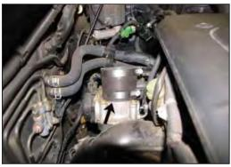
14. Install the supplied silicone hose (084016) onto the throttle body and secure with the supplied hose clamp.
