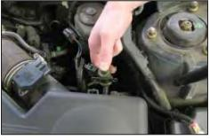
5. On vehicles not equipped with the "EVAP canister closed valve", install the supplied caplug onto the K&N® intake tube. Loosen the two upper air box mounting bolts, then remove the screw that secures the "EVAP canister closed valve" to the upper airbox as shown in the photograph.
