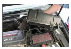
6. Release the clamp that secures the stock intake tube to the throttle body. Then, remove the factory intake tube/upper air box as shown in the photograph.
