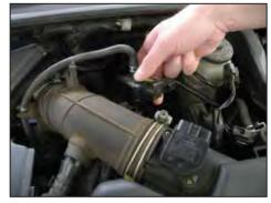
3. Remove the pulse width modulated (PWM) vacuum switching valve from the stock intake tube by gently pulling upwards until the PWM vacuum switching valve is released.
