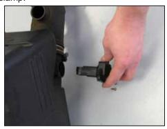
15. Remove the two screws that secure the mass air sensor into the stock air box; then, remove the mass air sensor.
