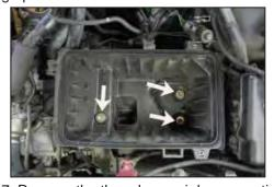
7. Remove the three lower air box mounting bolts; then, release the two wiring harness mounting clips which secure the wiring harness to the lower air box.
