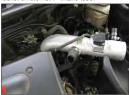
21. Install the K&N $^{\circledR}$  intake tube into the silicone (084016) hose on the throttle body; and align with the intake tube mounting bracket which was installed in step 13.
