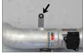
20. Install the provided grommet into the welded bracket on the  $K\&N^{\mbox{\scriptsize $B$}}$  intake tube.
