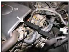
13. Install the intake tube mounting bracket (26651) onto the engine using the provided hardare as shown in the photograph.
