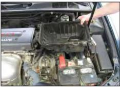
8. Remove the lower air box from it's place of attachment as shown in the photograph.
