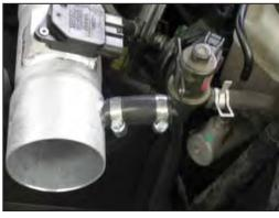
23. On vehicles not equipped with an "EVAP canister closed valve", install the "EVAP canister closed valve" into the silicone hose which was installed in step 19; secure with the provided hose clamp.
