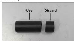
18. Cut the provided silicone hose (08415) hose from 2-3/8" (as supplied) to 1-3/4" long as shown in the photograph.
