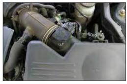
2. Disconnect the mass sensor electrical connection by depressing the center tab and gently pulling the harness away from the mass air sensor.
