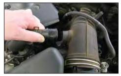
4. Compress and slide back factory hose clamp and remove the crank case vent hose/chamber from the stock intake tube as shown in the photograph.
