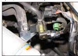
24. Install the pulse width modulated (PWM) switching valve into the grommet on the welded bracket on the intake tube as shown in the photograph.
