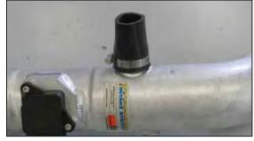
17. Install the provided silicone hose (084074) onto the  $K\&N^{\circledR}$  intake tube and secure with the provided hose clamp.
