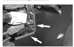
23. Cut the provided edge trim to size and place onto the heat shield as shown.
