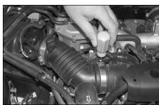
5. Loosen the hose clamp on the turbo charger inlet tube as shown.
