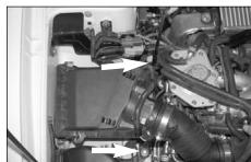
4. Loosen and remove the two bolts on the air cleaner as shown.
