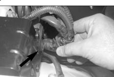
24. Unclip the wire harness from the inner fender bracket as some slack will be needed to reroute the mass air sensor electrical connection.
