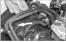
3. Unclip the coolant lines from the top of the air cleaner as shown.
