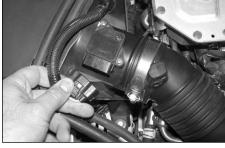
2. Disconnect the mass air sensor electrical connection as shown.
