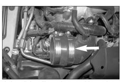
8. Install the silicone hose and hose clamps onto the turbo charger inlet tube as shown.
