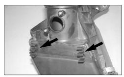
21. Remove the stock coolant clips from the stock air cleaner assembly as shown.
