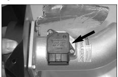
17. Install the mass air sensor into the K&N intake tube using the provided screws as shown above.
