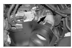
18. Install the complete air cleaner assembly into the vehicle and slide the intake tube into the silicone hose as shown above.
