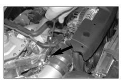
20. Tighten the hose clamp on the K&N intake tube as shown.
