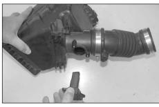
7. Remove the mass air sensor from the air cleaner as shown.
