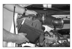
6. Remove the complete air cleaner assembly as shown.
