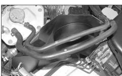
22. Install the stock coolant clips onto the two tabs on the heat shield, then clip the coolant lines onto the clips as shown.
