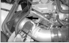
25. Reroute the mass air sensor electrical connection behind the heat shield and between the heat deflector plate and reconnect as shown.
