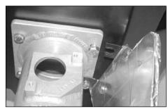
13. Using the remaining hex bolts install the heat deflector plate onto the intake tube flange as shown.
