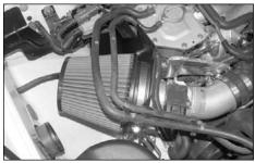
26. Install the K&N Filtercharger and secure using the provided hose clamp as shown.
