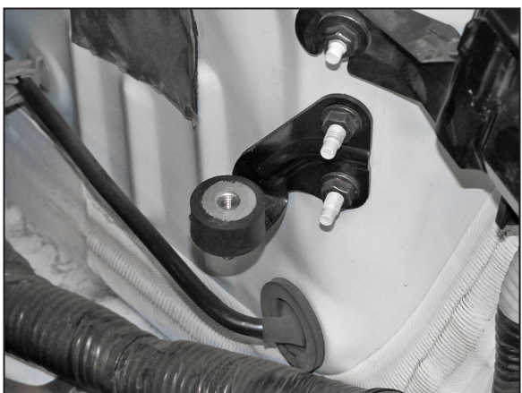
15. Install the remaining 1/2" long stud onto the upper air box mounting bracket as shown.
