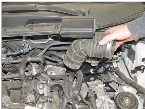
9. Loosen the hose clamp securing the intake hose to the throttle body and then remove the hose from the vehicle.
