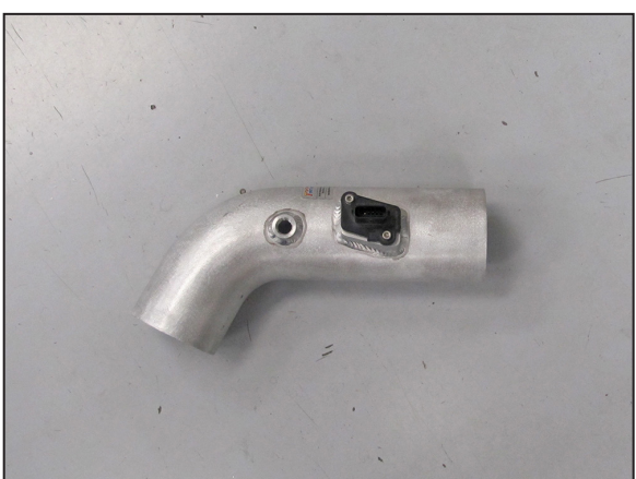
21. Install the mass air sensor into the K&N intake tube and secure with the provided hardware.
