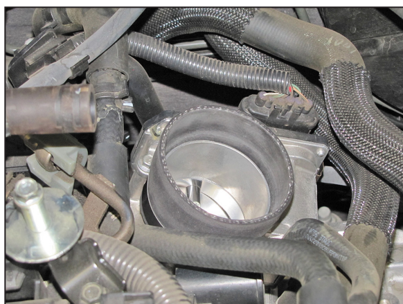
10. Install the coupling hose (084036) onto the throttle body and secure with the provided hose clamp.
