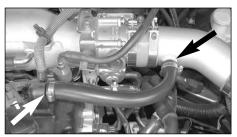
38. Install the provided vent hose onto the cam cover and the intake tube and secure with the provided hose clamps as shown.
