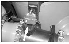
39. Reconnect the mass air sensor electrical connection as shown.
