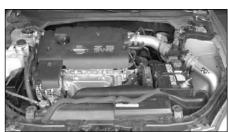
40. Re-install the engine cover with the four bolts that were removed in step 2.
