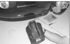
38. Install the filter onto the cold air tube from underneath the vehicle as shown.
