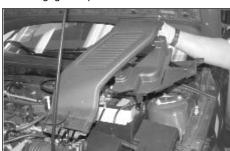
4. Slide the battery cold air vent backwards and remove from the engine compartment as shown.
