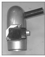
26. Install the mass air sensor into the intake tube using the provided hardware as shown.
