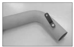
33. Install the provided bracket onto the cold air tube using the provided hardware as shown.
