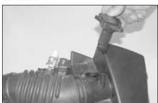
14. Remove the mass air sensor from the air cleaner cover as shown.
