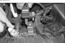
Remove the switch/sensor from the air cleaner cover as shown.
