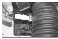
15. Remove the plastic clip from the crank case vent on the stock intake tube as shown.
