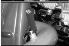
36. Secure the bracket to the rubber mounted stud using the provided hardware as shown. NOTE: On the '06 Mazda 5 models, secure the bracket with the stock air box mounting stud removed earlier into the resonator threaded hole as shown.
