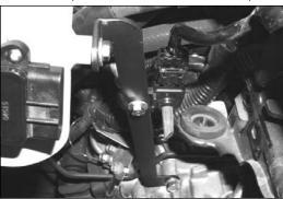
28. Secure the switch from step 7 to the bracket using the provided hardware as shown.
