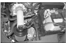
45. This K&N Typhoon kit is designed for use in two different configurations. In the case of inclement weather, the cold air tube can be removed and the filter can be clamped onto the short ram tube located in the engine compartment as shown above, to avoid the possibility of ingesting water into the engine.
