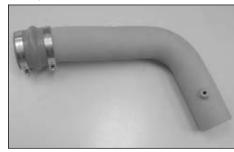
32. Install the silicone hose and hose clamps onto the cold air tube as shown.
