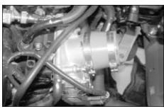
24. Install the silicone hose and hose clamps onto the throttle body as shown.
