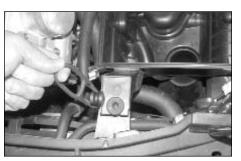
11. Remove the rubber retainer from the core
