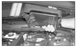
2. Unclip the battery cover and remove, then, disconnect the negative battery cable.
