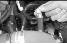
29. Install the crankcase vent from step 18 into the silicone hose on the intake tube as shown.
