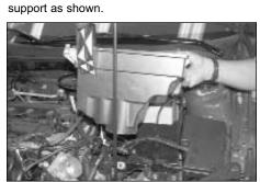
12. Remove the lower air cleaner assembly as shown.
