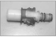
18. Slide the plastic clip from step 15 back onto the crank case vent as shown.
