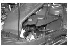
42. Slide the vent into the core support and line up the other end with the battery box and secure with plastic rivet.
