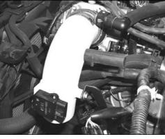
27. Install the K&N intake tube into the silicone hose at the throttle body and align with the mounting bracket. Secure the tube with the provided hardware and hose clamp.
