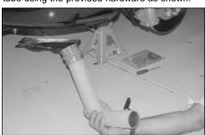
34. From underneath the vehicle install the cold air tube as shown.
