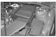
43. Reconnect the negative battery cable, then, reinstall the battery cover as shown.
