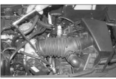
8. Loosen the hose clamp at the throttle body a shown.
