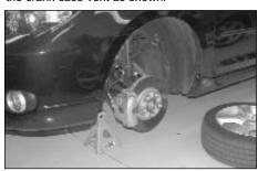
19. Raise the vehicle up and support it with jack stands, then, remove the front tire as shown.
