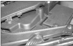
3. Disengage the plastic rivet as shown.
