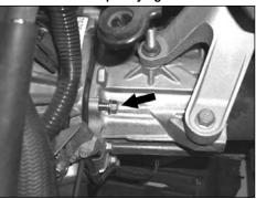
23a. On vehicles equipped with a manual transmission, remove the transmission bellhousing bolt shown.
