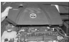
Pull firmly upwards to remove the engine cover as shown
