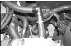
30. Reconnect the crankcase vent as shown. NOTE: For best fit, trimming of the silicone hose may be necessary.
