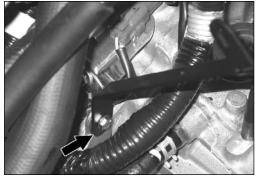
23. On vehicles equipped with an automatic transmission, attach the tube mounting bracket (#06479) onto the transmission control cable bracket using the provided hardware.
