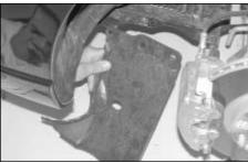
20. Remove the four bolts and one plastic rivet from the inner valance then, remove the valance as shown
