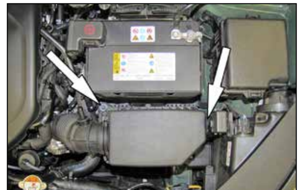
6. Remove the two bolts securing the air box.
