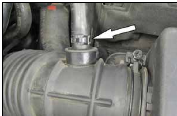
4. Release the spring clamp securing the crank case vent hose to the intake tube and then disconnect the crank case vent hose.
