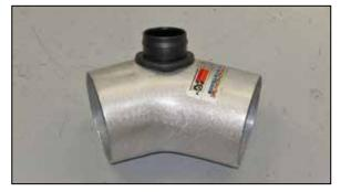
13. Install the provided quick disconnect fitting into the grommet installed into the K&N® intake tube.
