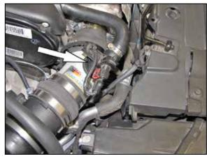
19. Connect the Pressure sensor to the guick disconnect fitting installed into the K&N® intake tube.
