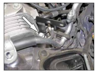
7. Install the heat shield mounting bracket (083149) onto the engine mount and secure it with the bolt removed in the previous step.
