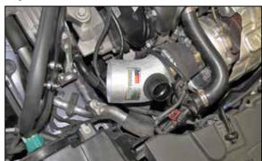
14. Install the K&N® intake tube into the coupler at the turbo but do completely tighten at this time.
