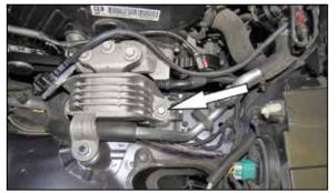
6. Remove the motor mount bolt show.
