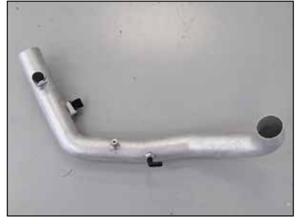
18. Install the 90° npt fitting into the K&N intake tube as shown. NOTE: Plastic NPT fittings are easy to cross thread. Install the vent fitting "hand" tight, then turn it two complete turns with a wrench.
