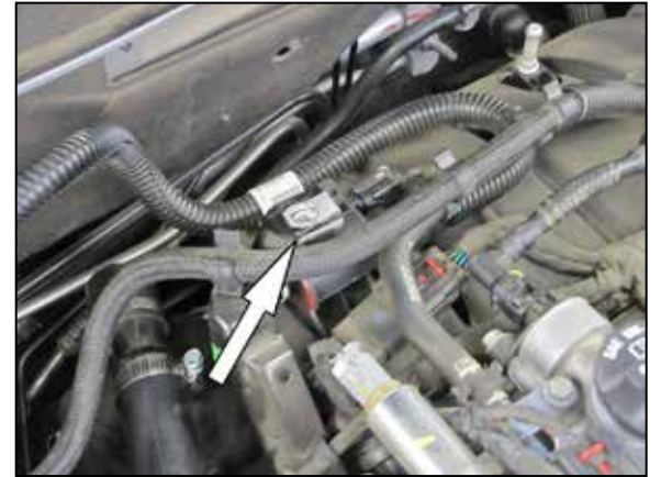
19. Remove the clip nut from the plenum mounting bracket.
