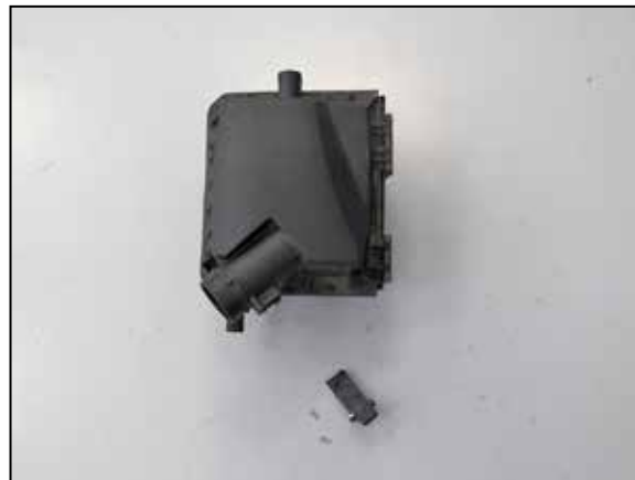
15. Remove the two screws securing the mass air sensor and then remove the mass air sensor from the air box.
