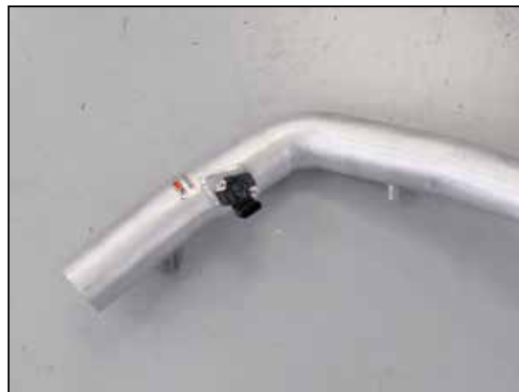
16. Install the mass air sensor into the K&N intake tube as shown.
