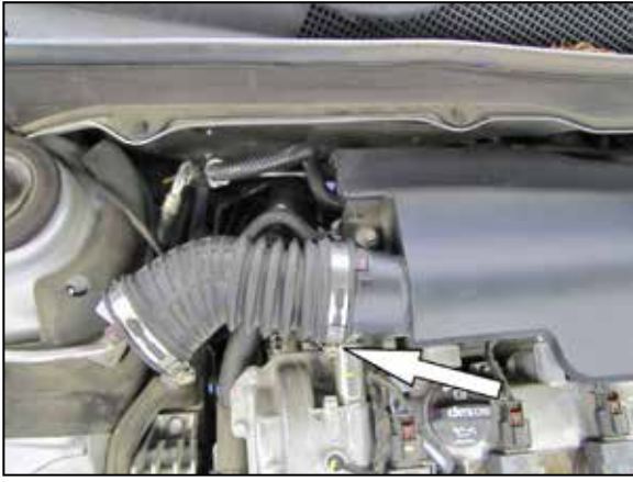
7. Remove the bolt shown securing the intake plenum to the engine.
