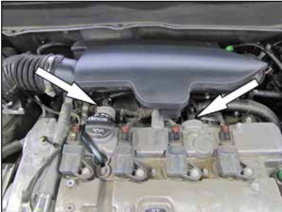
9. As the intake plenum is being lifted off, release the locking tabs on the two crank case vents and disconnect the crank case vents from the valve cover. Once the intake plenum is free, remove it from the vehicle.
