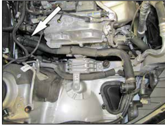
12. On vehicles equipped with air injection, cut the clamp at the air injection hose union and then separate the air injection hose and remove the loose section from the vehicle.
