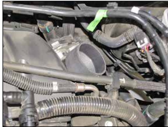
14. Install the provided coupling hose (08440) onto the throttle body and secure with provided hose clamp.
