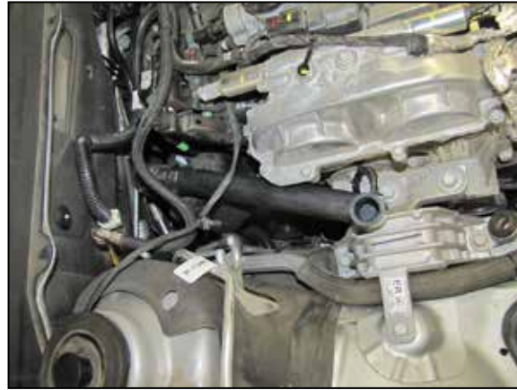
13. On vehicles equipped with air injection, install the provided air injection hose (08479) onto the factory union and secure with provided hose clamp. NOTE: Do not completely tighten at this time.
