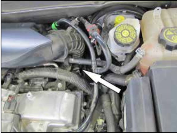
8. Loosen the hose clamp securing the intake tube to the throttle body.
