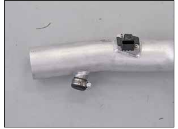
17. On vehicles that are not equipped with air injection, install the provided cap plug onto the air injection port and secure with the provided hose clamp.
