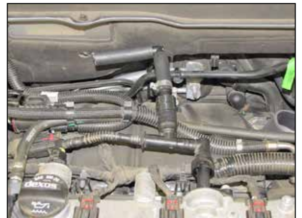
21. Install the crank case vent hose assembly into the factory quick disconnect fitting and then rotate the assembly back towards the fire wall as shown.
