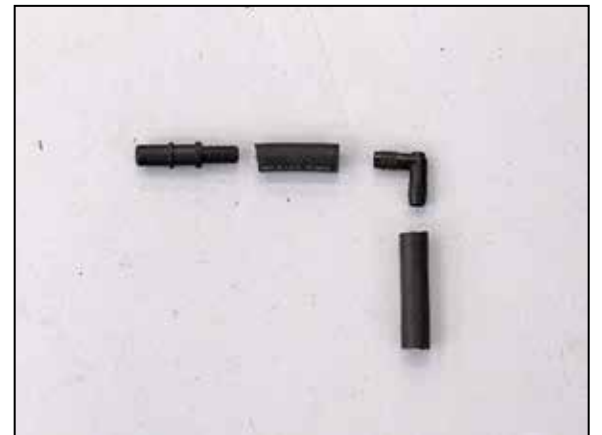
20. Assemble the two provided crank case vent hoses, quick disconnect fitting and 90° hose mender as shown.
