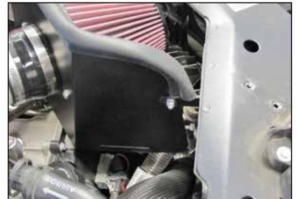
24. Secure the heat shield to the mounting bracket with the hardware provided.
