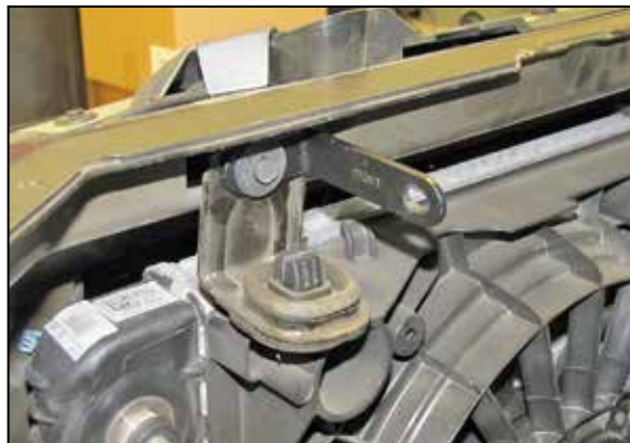
20. Install the provided "L" bracket (07093) onto the radiator mount and secure with the factory bolt removed in step #19.
