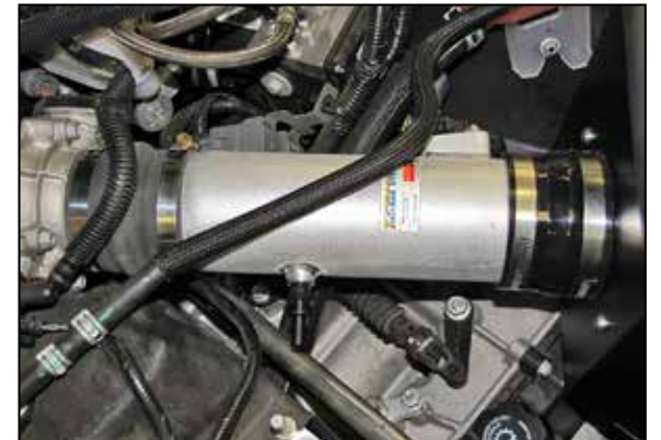
23. Install the K&N® intake tube into the hose at the throttle body and align the tube with the filter adapter. Slide the hose into position and secure with the provided hose clamps.
