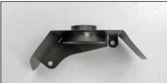
14. Install the filter adapter into the heat shield and secure with the provided hardware.
