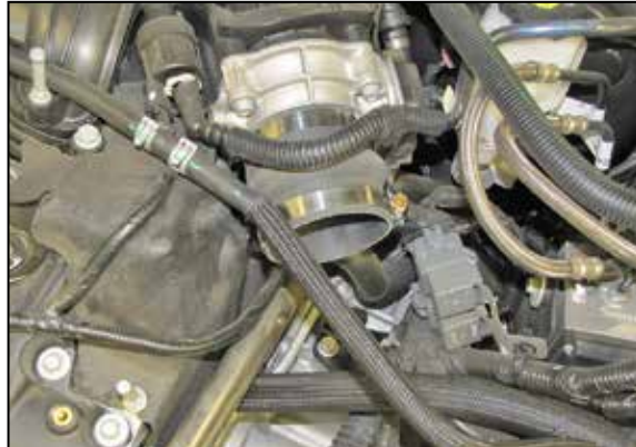
18. Install the provided hump hose (08696) onto the throttle body and secure with the provided hose clamp.
