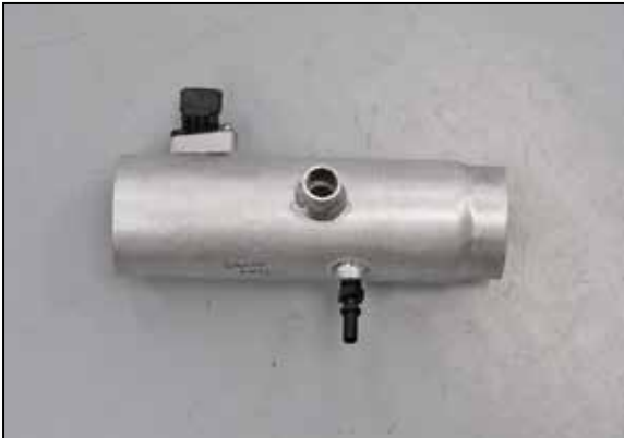
13. Install the provided quick disconnect fitting into the K&N intake tube as shown. NOTE: Plastic NPT fittings are easy to cross thread. Install the vent fitting "hand" tight, then turn it two complete turns with a wrench.
