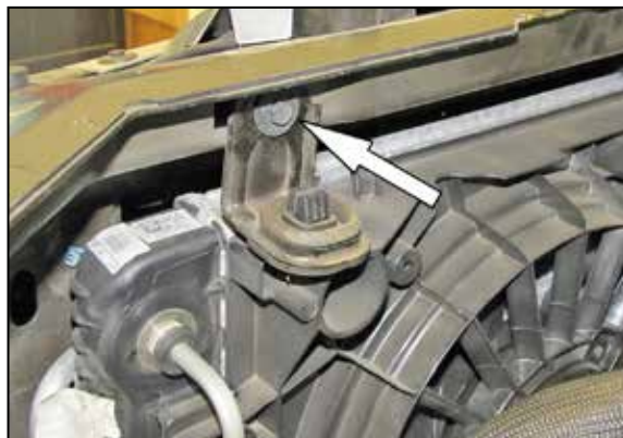
19. Remove the bolt shown that secures the radiator mount to the core support.
