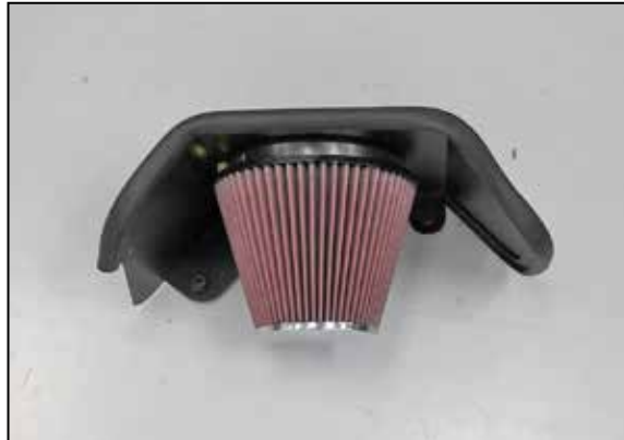
17. Install the air filter onto the filter adapter and secure with the provided hose clamp.
