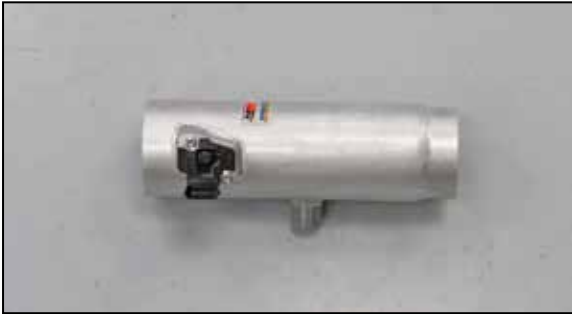
12. Install the mass air sensor and secure with the provided hardware.
