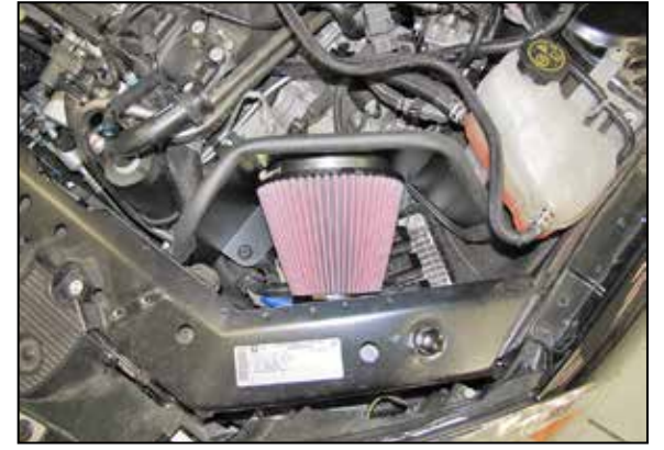
21. Install the heat shield assembly into the vehicle so the mounting grommets set onto the mounting studs.
