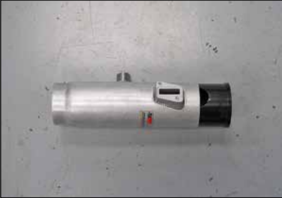
11. Install the mass air insert into the K&N® intake tube so that the hole in the insert aligns with the mass air location in the tube.
