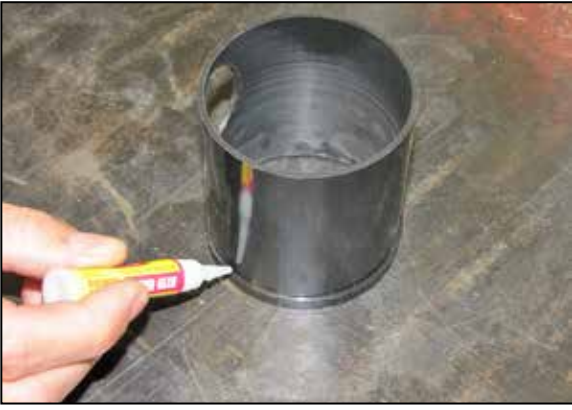
10. Apply several drops of the provided glue to the mass air insert as shown.
