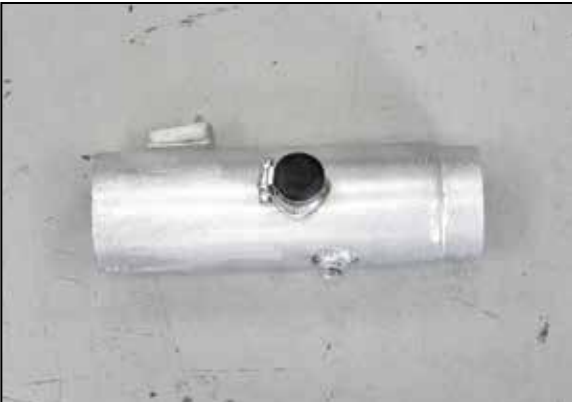
13a. On vehicles that are not equipped with air injection, install the provided cap onto the fitting and secure with the provided hose clamp.
