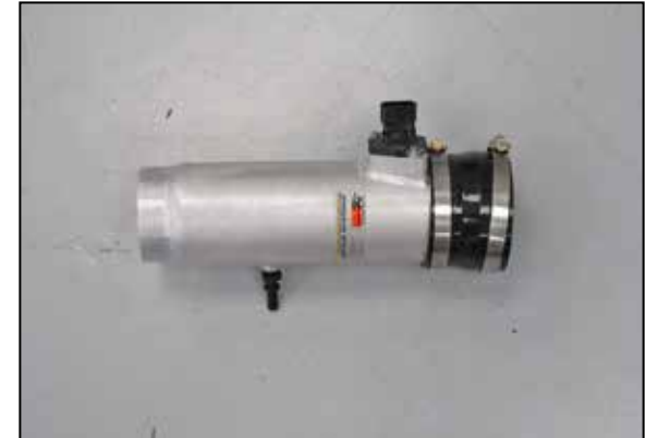
22. Install the provided hose (08496) onto the intake tube as far as it will slide on, do not tighten at this time.
