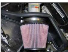
19. Install the K&N® air filter onto the filter adapter and secure with the provided hose clamp.
