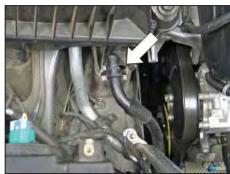
3. Remove the air box drain pipe from the front of the air box.
