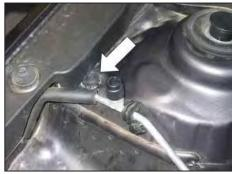
9. Remove the plastic plug and then install the inserted nut into the strut tower as shown.
