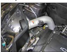
17. Set the intake assembly into position so the intake tube is inserted into the silicone hose, the rubber insert mounts into the front lower air box mount and the rubber mounted stud is attached to the heat shield.
