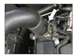
4. Loosen the hose clamp that secures the factory intake tube to the throttle body and then disconnect the intake tube from the throttle body.
