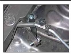
10. Install the heat shield bracket assembly onto the strut tower as shown using the provided hardware.
