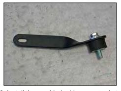
8. Install the provided rubber mounted stud onto the provided heat shield bracket (07945) as shown.
