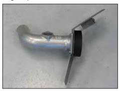
13. Install the filter adapter and K&N® intake tube onto the heat shield as shown using the provided hardware and gaskets.
