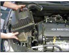
5. Lift up the air box assembly to dislodge it from the mounting grommets; then remove the air box assembly from the vehicle.
