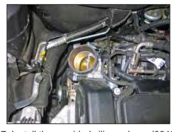
7. Install the provided silicone hose (084014) onto the throttle body and secure with the provided hose clamp.
