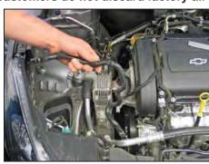
6. Remove the air box drain pipe from the vehicle. NOTE: The drain pipe is connected to the inner fender by two plastic clips that will need to be removed or clipped.
