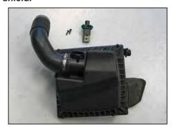
14. Remove the two screws securing the mass air sensor into the factory air box; remove the sensor from the air box.
