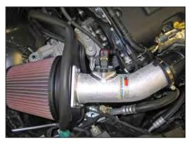
18. Connect the mass air sensor electrical connec-
