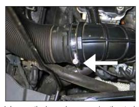
4. Loosen the hose clamp securing the stock intake tube to the intake elbow.
