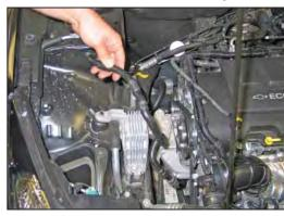
6. Unhook the two clips that secure the airbox drain tube to the inner fender, and then remove the drain tube from the vehicle.
