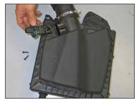
Remove the two screws that secure the mass air sensor to the factory airbox and then remove the mass air sensor from the airbox.
