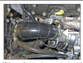
15. Loosen the hose clamp securing the intake elbow to the throttle body so that the intake elbow position can be adjusted.
