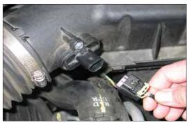
2. Release the locking and then disconnect the mass air sensor electrical connector.
