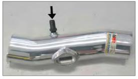
16. Install the provided 1/4npt vent fitting into the K&N intake tube as shown.
