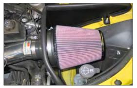
22. Install the K&N air filter and secure with the provided hose clamp.
