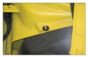
13. Install the provided rubber fender washer onto the outward air box mounting stud.
