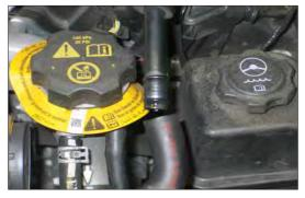
4. Disconnect the crank case vent hard line from the 90\* connector hose on the factory intake tube.
