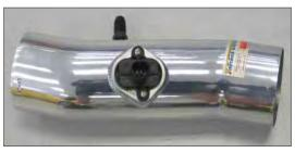
18. Install the mass air sensor into the K&N intake tube and secure with the provided hardware. **NOTE: The o-ring seal provides a very tight seal, be sure the o-ring is properly seated as the sensor is being installed.**  23. Reconnect the mass air sensor electrical connection.
