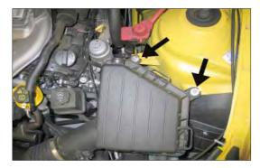
6. Remove the two nuts shown securing the factory air box to the inner fender.
