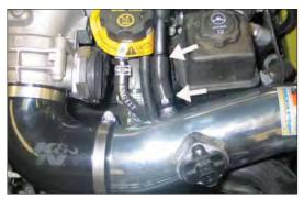
21. Install the provided silicone hose onto the factory crank case vent tube and then connect the open end onto the vent fitting installed into the K&N intake tube.
