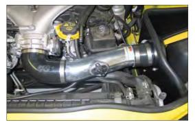
20. Install the K&N intake tube assembly into the silicone hose at the filter adapter and then onto the throttle body, align for proper fit and then secure with the provided hose clamps.
