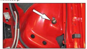
11. Install the provided rubber mounted stud onto the inner fender at the factory air box mounting location.
