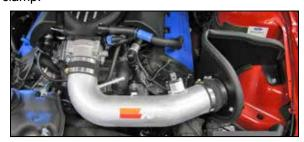
18. Install the K&N® intake tube into the hose at the filter adapter and then into the hose at the throttle body, adjust the tube for best fit and then secure with the provided hose clamp.
