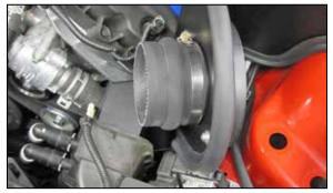
17. Install the provided coupling hose (08699) onto the filter adapter and secure with the provided hose clamp.
