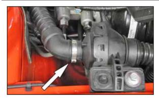
7. Cut the clamp securing the engine sound tube to the drum and the remove the engine sound tube from the vehicle. Install the provided cap plug onto the drum.
