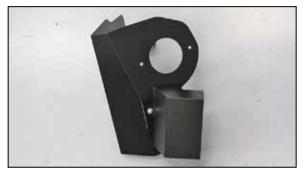
8. Install the provided fresh air duct onto the heat shield and secure with the provided hardware.
