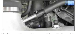
19. Connect the crank case vent hose to the quick connect fitting on the K&N® intake tube.
