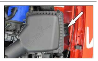
5. Remove the bolt securing air box to the inner fender.
