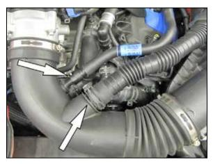
3. Disconnect the crank case vent hose and engine sound tube from the intake tube.
