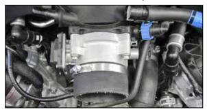
16. Install the provided coupling hose (08698) onto the throttle body and secure with the provided hose clamp.
