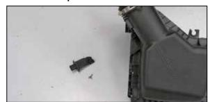
14. Remove the Mass air sensor from the factory air box.
