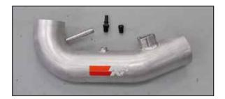
13. On vehicle equipped with an EVAP hose, install the provided quick disconnect fitting into the K&N® intake tube. On vehicles not equipped with an EVAP hose, install the provided plug into the K&N® intake tube.
