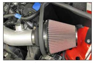
20. Install the K&N® air filter onto the filter adapter and secure with the provided hose clamp.
