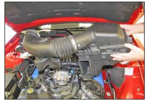
6. Disconnect the intake tube from the throttle body then remove the complete intake system from the vehicle
