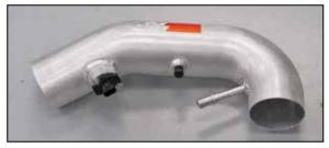
15. Install the mass air sensor into the K&N<sup>®</sup> intake tube and secure with the hardware provided.
