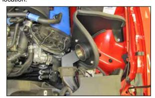
12. Install the heat shield assembly onto the inner fender and into the fresh air intake. Secure the heat shield with the hardware provided.
