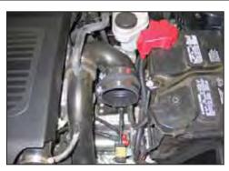
15. Install the provided silicone hump hose (08699) onto the factory inlet tube as shown and secure with the provided hose clamp.
