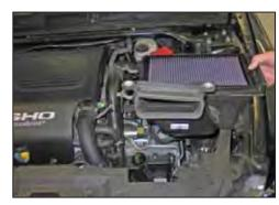
7. Lift up the airbox and remove it from the vehicle.
