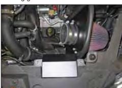
14. Install the provided fresh air scoop onto the core support and then secure the scoop to the core support and heat shield with the provided hard-
