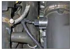
3. Disconnect the inlet air temperature sensor electrical connection and unhook the wiring harness from the upper airbox.
