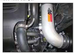
19. Reconnect the inlet air temperature sensor electrical connection.
