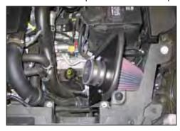
13. Install the heat shield/filter assembly into the vehicle so the mounting studs insert into the airbox mounting grommets
