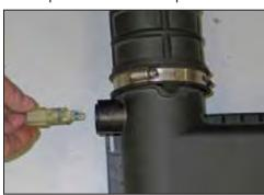
16. Release the locking tab on the inlet air temperature sensor and rotate counter clockwise to remove it from the factory airbox.
