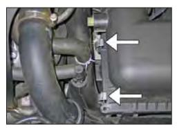
4. Release the two upper airbox retaining clips.
