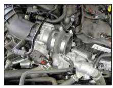
9. Install the provided silicone hose (08696) onto the throttle body and secure with the provided hose clamp as shown.
