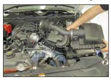
6. Remove the upper air box/tube assembly from the vehicle.
