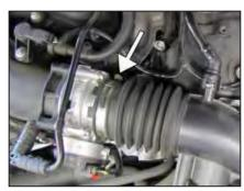
3. Loosen the hose clamp that secures the factory intake tube to the throttle body.
