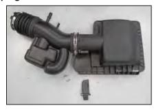
17. Remove the two screws securing the mass air sensor into the factory air box and then remove the mass air sensor.
