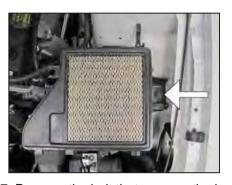
7. Remove the bolt that secures the lower air box to the inner fender shown.
