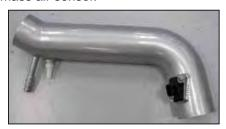
18. Install the mass air sensor into the K&N® intake tube and secure with the provided hardware.
