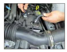
4. Release the locking tab securing the crank case vent hose to the intake tube, then disconnect the crank case vent hose and the EVAP hose from the factory intake tube.
