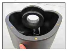
11. Install the K&N® filter adapter into the K&N® air box and secure with the provided hardware.
