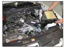
8. Remove the lower air box housing from the vehicle.
