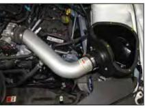
19. Install the K&N® intake tube into the silicone hose at the throttle body and then into the silicone hose on the filter adapter, secure the intake tube with the provided hose clamps.
