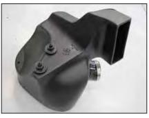
14. Install the air box mounting grommets onto the mounting studs installed onto the K&N® air box during step #10.
