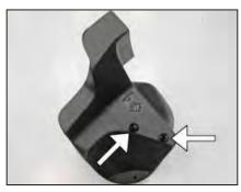
10. Install the two provided mounting studs to the bottom of the K&N® air box as shown and secure with the provided hardware.
