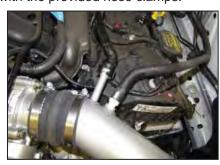
20. Connect the crank case vent hose and EVAP hose to the K&N® intake tube as shown. NOTE: Vehicles not equipped with an EVAP vent line should have this port plugged with the provided 1/4 npt plug.
