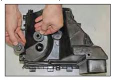
13. Remove the factory air box mounting grommet from the factory lower air box housing.
