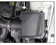
5. Release the two clips that secure the upper air box to the lower air box housing.
