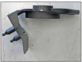
11. Install the filter adapter onto the heat shield and secure with the provided hardware.
