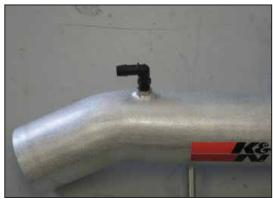
16. Install the provided  $90^{\circ}$  npt vent fitting into the K&N® intake tube as shown.
