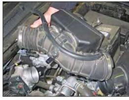
6. Remove the stock intake tube from the vehicle.
