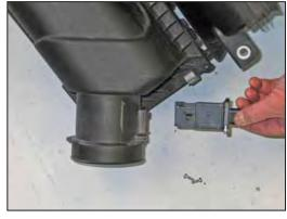
14. Remove the mass air sensor mounting bolts, then remove the mass air sensor from the factory airbox.
