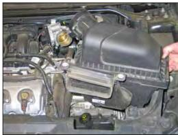
8. Lift up the airbox assembly to dislodge it from the mounting grommets and then remove the airbox from the vehicle.
