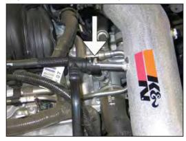
20. Connect the crankcase vent hose to the quick connect fitting on the K&N® intake tube.
