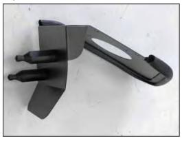
10. Install the heat shield mounts onto the heat shield and secure with the provided hardware.
