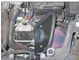
13. Install the heat shield/filter assembly into the vehicle so that the mounts snap into the factory airbox mounts.
