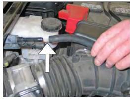
3. Disconnect the EVAP hose from the check valve connection.
