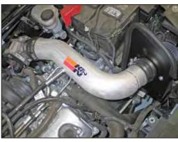
19. Install the K&N® intake tube assembly into the hose at the throttle body and then onto the filter adapter and secure with the provided hose clamp.
