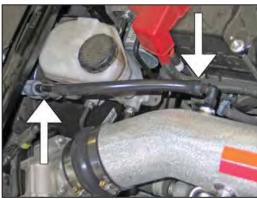
21. Connect the provided EVAP hose onto the 90° vent fitting installed in the K&N® intake tube, then connect the open end to the EVAP check valve as shown.
