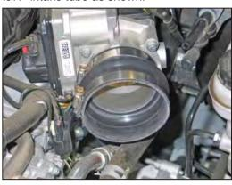
17. Install the provided silicone hose (084079) onto the throttle body and secure with the provided hose clamp.
