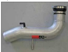
18. Install the provided silicone hose (084091) onto the K&N® intake tube as shown and secure with the provided hose clamp.
