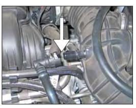
4. Release the grey locking tab and then disconnect the crankcase vent line from the intake tube.
