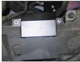
23. Install the fresh air intake scoop into position and secure to the heat shield and core support with the provided hardware.
