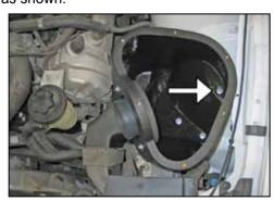
15. Set the K&N® airbox into position on the inner fender and secure to the factory mounting location with the hardware provided.
