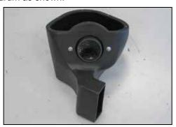
11. Install the filter adapter into the K&N® airbox and secure with the provided hardware.
