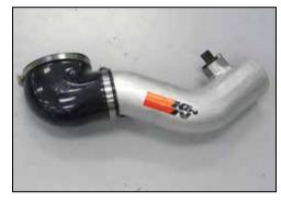
20. Install the 90° silicone hose onto the K&N® intake tube as shown. Do not tighten the hose clamp at this time.
