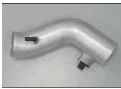
18. Install the  $90^{\circ}$  vent fitting into the K&N® intake tube as shown.
