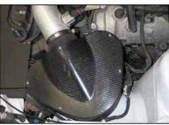
27. Connect the mass air harness to the vehicle harness, routing the mass air harness around the  $K\&N^{\circledcirc}$  airbox. Connect the mass air harness to the mass air sensor.
