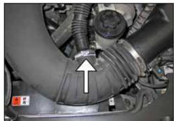
3. Release the spring clamp that secures the engine pulse hose to the factory intake tube, and then disconnect the engine pulse hose from the intake tube.
