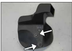
14. Install the two airbox mounting grommets to the mounting studs installed onto the  $K\&N^{\otimes}$  airbox as shown.
