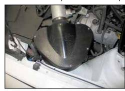
25. Install the airbox lid onto the airbox and secure with the provided hardware.
