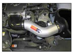
22. Install the K&N® intake tube assembly into the silicone hose on the filter adapter, and then into the 90° hose attached to the throttle body. Adjust the tube and hose for proper fit, then tighten the hose clamps.
