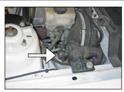
10. Install the provided cap plug onto the pulse drum as shown.
