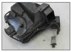
16. Remove the two screws securing the mass air sensor and then remove the mass air sensor from the factory airbox.
