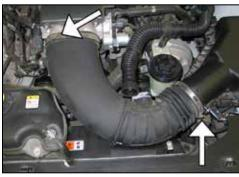
5. Loosen the two hose clamps that secure the intake tube to the throttle body and airbox, and then remove the intake tube from the vehicle.
