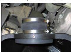
19. Install the silicone hump hose (08699) onto the filter adapter and secure with the provided hose clamp.
