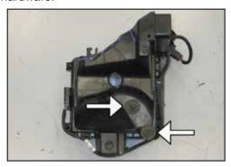
13. Remove the two airbox mounting grommets from the factory airbox.
