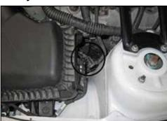
2. Disconnect the mass air sensor harness electrical connection at the rear of the airbox.
