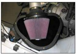
24. Install the K&N® air filter onto the filter adapter and secure with the provided hose clamp.
