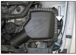
6. Remove the bolt shown that secures the factory airbox to the fender well.
