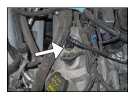
4. Release the locking tab and then disconnect the crankcase vent tube from the valve cover.
