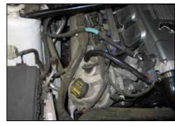
23. Connect the crankcase vent hose to the vent port on the valve cover.
