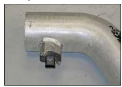
17. Install the mass air sensor into the K&N $^{\!0}$  intake tube and secure with the provided hardware.
