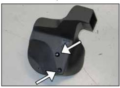
12. Install the two provided mounting studs onto the bottom of the K&N® airbox using the provided hardware.
