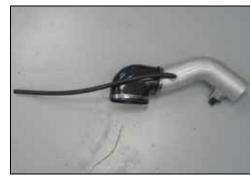
21. Install the provided crankcase vent hose onto the 90° fitting installed into the K&N® intake tube.
