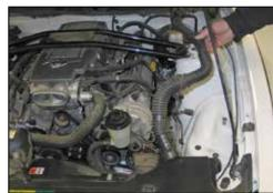
9. Remove the engine pulse hose from the vehicle.
