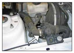
8. Cut the hose clamp securing the engine pulse hose to the engine pulse drum.
