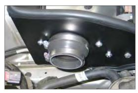
16. Install the provided step hose (084093) onto the filter adapter and secure with the provided hose clamp.
