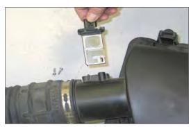
17. Remove the two screws which secure the mass air sensor and then remove the mass air sensor from the stock air box.
