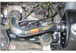
19. Install the K&N® intake tube into the silicone hose on the filter adapter and then into the silicone hose at the throttle body. Secure the intake tube with the provided hose clamps.
