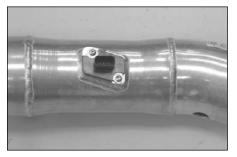
16. Install the mass air sensor into the K&N intake tube with the provided hardware as shown.
