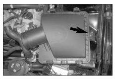
5. Remove the air box mounting bolt shown.
