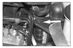
13. Remove the radiator fan shroud mounting bolt shown. NOTE: This bolt will not be reused.
