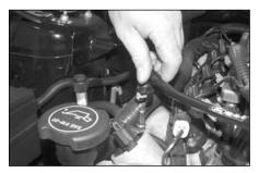
3. Rotate the green locking tab clockwise and then disconnect the crank case breather hose from the valve cover as shown.
