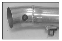
17. Install the grommet provided into the K&N intake tube as shown.
