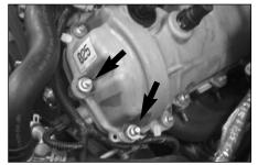
7. Remove the two valve cover bolts shown. **NOTE: These bolts will be reused.**
