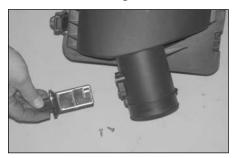
15. Remove the mass air sensor from the factory air box with the T20 "TORX" wrench provided.
