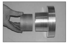
23. Place the Hydrocarbon trap into the filter adapter as shown.
