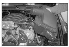
6. Remove the air box assembly as shown.
