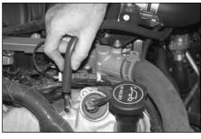
21. Install the crank case vent hose mender into the grommet installed in the K&N intake tube and then onto the valve cover as shown.
