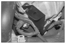
9. Install the tube-mounting bracket onto the valve cover as shown and secure with the stock hardware removed in step #7.
