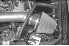
26. Install the air filter assembly onto the K&N intake tube as shown and secure with the provided hose clamp.
