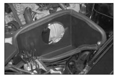
14. Install the heat shield and secure with the provided hardware as shown.
