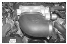
18. Install the silicone hose (084094) onto the throttle body with the provided hose clamp as shown.
