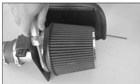
20. Install the K&N Filtercharger onto the filter adapter and secure with the provided hose clamp as shown.
