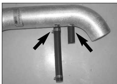
17. Install the provided hoses from the previous step onto the K&N intake tube and secure with the provided hose clamps as shown.
