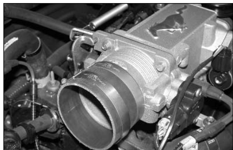
15. Install the provided silicone hose and hose clamps onto the throttle body as shown.
