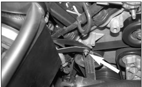
22. Slide the brackets onto the stud from step 11 and secure with the factory nut.
