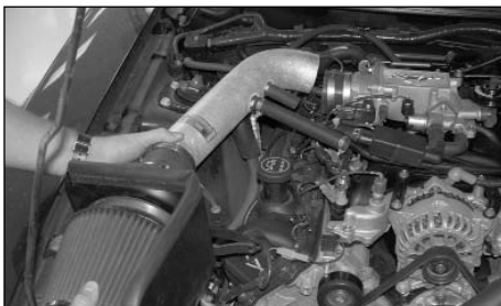
18. Install the provided silicone step hose and hose clamps onto the K&N intake tube as shown.
