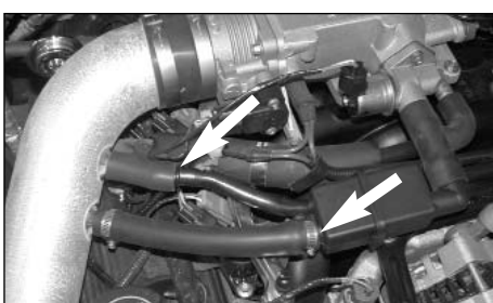
23. Reconnect the vent hoses to the K&N intake tube as shown and tighten hose clamps.
