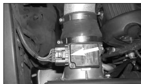
24. Reconnect mass air sensor electrical connection as shown.
