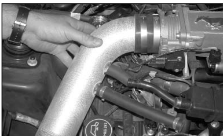
21. Install the complete K&N intake assembly into the vehicle and slide the tube into the silicone hose on the throttle body as shown.
