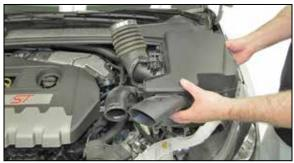
5. Remove the air box from the engine compartment.
