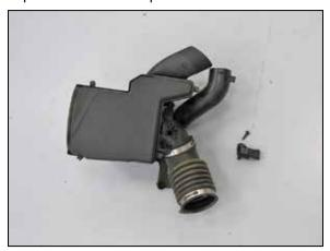
16. Remove the pressure sensor from the factory air box as shown.
