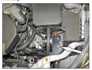
11. Install the heat shield assembly into the engine compartment and secure it to the rubber mounted stud with the provided hardware.
