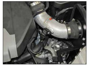
19. Reconnect the pressure sensor electrical connection.
