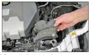
6. Remove the fresh air duct from the core support as shown.
