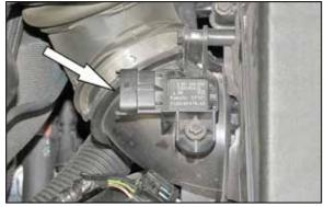
2. Disconnect the pressure sensor electrical connection.
