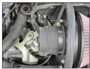
15. Install the provided coupling hose #084055 onto the filter adapter as shown and secure with the provided hose clamp.
