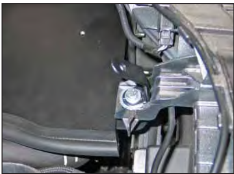
18. Using the provided hardware, secure the provided bracket (083161) to the fresh air intake scoop mount and the rubber mounted stud on the heat shield base. NOTE: The provided fender washer from the previous step should be placed between the bracket and the fresh air intake scoop mount.
