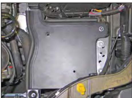
16. Set the heat shield base into position on the air box mounts.
