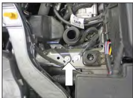
10. Remove the bolt shown securing the intake silencer to the inner fender; lift up to remove the intake silencer from the vehicle.
