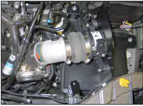
27. Install the K&N intake tube into the silicone hose on the throttle body, then align the heat shield and secure with the provided hardware. Align the intake tube and secure with the provided hose clamps.
