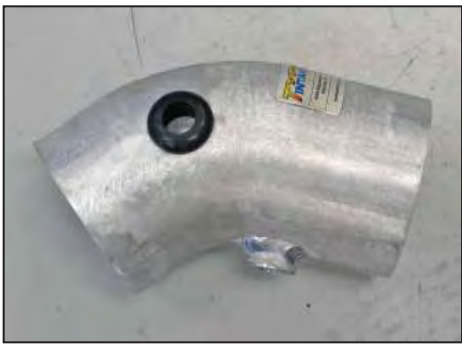
24. Install the provided 1.0"OD grommet into the K&N intake tube as shown.
