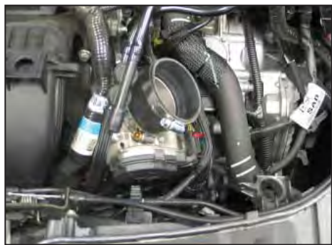
11. Install the provided silicone hose (084016) onto the throttle body and secure with the provided hose clamp.
