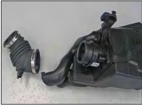
20. Loosen the hose clamp that secures the factory intake tube to the mass air sensor housing and then remove the hose from the mass air housing.
