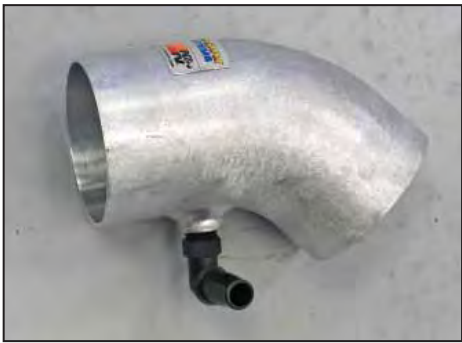
25. Install the 90° vent fitting into the K&N intake tube as shown.
