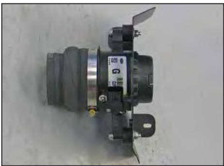
23. Install the provided hump hose (08421) onto the mass air sensor as shown and secure with the provided hose clamp.
