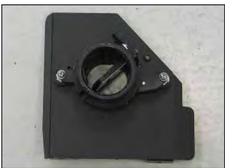
22. Secure the mass air sensor housing to the rubber mounted studs on the heat shield as shown using the provided hardware.
