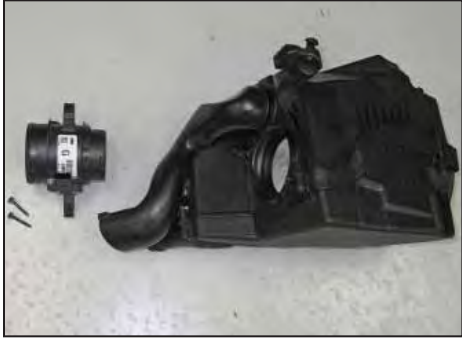
21. Remove the two bolts securing the mass air sensor housing to the air box; separate the mass air housing from the air box.
