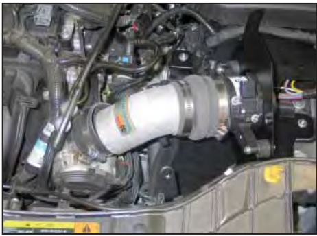
26. Install the K&N intake tube completely into the silicone hump hose and then set the complete assembly onto the heat shield base.
