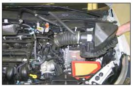
6. Remove factory intake hose and airbox lid from the vehicle.
