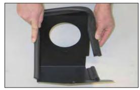
16. Attach long edge trim to heat shield as shown. **NOTE: Some trimming maybe necessary.**
