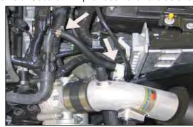
24. Install provided silicone hose onto the EVAP valve with provided hose clamp then onto  $90^{\circ}$  fitting on K&N® intake tube.
