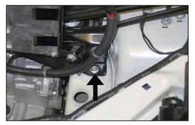
10. Remove bolt shown securing the ECU bracket. **NOTE: bolt will be reused.**
