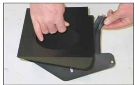
15. Attach short edge trim to heat shield as shown. **NOTE: Some trimming maybe necessary.**
