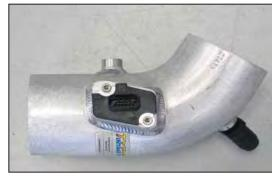
22. Install mass air sensor into K&N® intake tube and secure with the provided hardware as shown.
