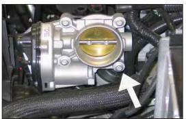
11. Remove bolt shown from throttle body. **NOTE: bolt will be reused.**
