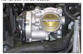
12. Install tube mounting bracket (083136) onto the throttle body using bolt removed from the previous step.
