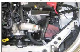
26. Install the K&N® filter onto K&N® intake tube secure with provided hose clamp as shown.
