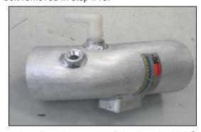
19. Install 90 degree vent fitting into the K&N<sup>®</sup> intake tube as shown.
