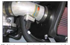
27. Attach mass air extension harness onto factory harness and connect the other end to the mass air sensor electrical connector.
