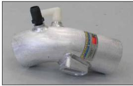
20. Install the 5/8" vent fitting into the  $K\&N^{\rm @}$  intake tube as shown.
