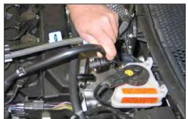
3. Release the locking tab and then disconnect the crankcase vent line from the rear of cam cover as shown
