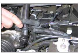
4. Remove EVAP hose from the EVAP valve as shown.
