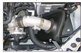
23. Install K&N® intake tube into silicone hose and aligning with tube mounting bracket and heat shield. Secure with provided hardware as shown.
