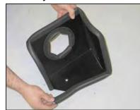
14. Install the long edge trim onto the heat shield as shown.
