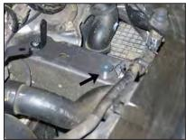
16. Place the heat shield spacer and fender washer
