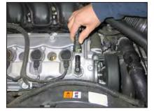
3. Disconnect the crankcase vent hose from the valve cover port as shown.
