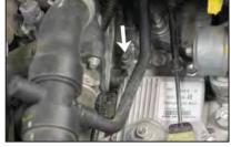
11. Remove the ground strap mounting bolt shown from the transmission.
