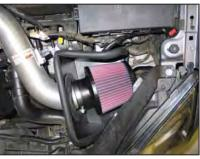
23. Install the K&N<sup>®</sup> air filter and secure with the provided hose clamp.
