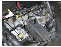
15. Install the heat shield mounting bracket (070602) onto the inner frame rail using the provided hardware as shown.
