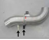
19. Install the two provided  $1\!\!\!/ "NPT$  fittings into the  $K\&N^{\circledast}$  intake tube as shown.
