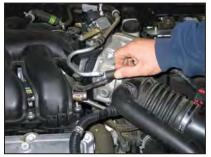
4. Disconnect the EVAP vent hose from the tube as shown.
