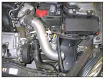
20. Install the K&N<sup>®</sup> intake tube into the silicone hose at the throttle body and align with the mounting bracket installed in step #12. Secure the intake tube with the hose clamp and hardware provided.
