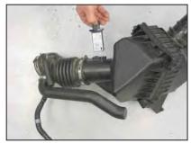
9. Remove the two screws which retain the mass air sensor and then remove the mass air sensor from the airbox.
