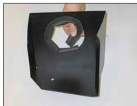
13. Install the short edge trim into the hole of the heat shield as shown.
