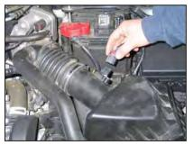
2. Disconnect mass air sensor electrical connection.
