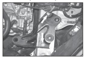
9. Remove the two bolts that fasten the air box mounting bracket to the inner fender, then remove the mounting bracket.
