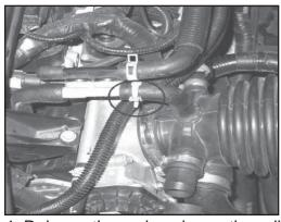
4. Release the spring clamp, then disconnect the solenoid valve hose from the stock plastic fitting.
