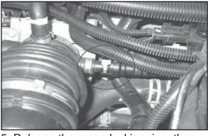
5. Release the green locking ring, then disconnect the crank case vent hose from the stock intake tube
