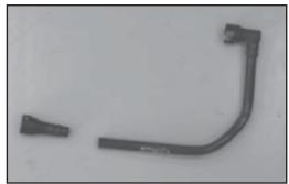
12. Disconnect the crank case vent hose from the valve cover, remove it, and place it on a surface suitable for cutting. Using a a razor blade or knife; cut the crank case vent hose as shown.
