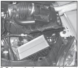
7. Release the three upper air box retaining clips, then remove the upper air box and intake tube assembly.
