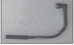
13. Install the supplied silicone vent hose onto the cut end of the stock crank case vent hose.
