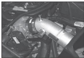
20. Install the K&N intake tube into the silicone hose (08440) and align the intake tube fastening location with the intake tube mounting bracket (06491.) Fasten using the provided hose clamp and mounting bracket hardware.
