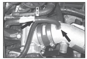
22. Connect the provided silicone solenoid valve hose to the stock fitting and K&N intake tube fitting.
