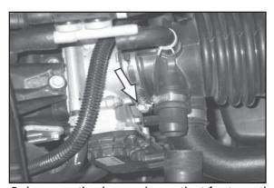
6. Loosen the hose clamp that fastens the stock intake tube to the throttle body.
