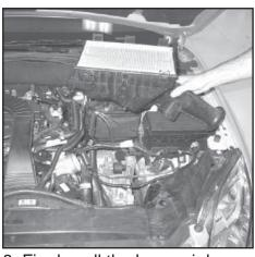
8. Firmly pull the lower air box upwards to dislodge it from the mounting grommets; remove the lower air box.
