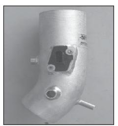
11. Install the mass air sensor into the K&N intake tube using the provided hardware.
