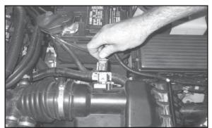
2. Release the red locking clip, then disconnect the mass air sensor electrical connection.
