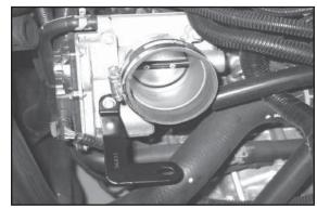
19. Install the intake tube mounting bracket and fasten using the factory bolt removed in step # 18.
