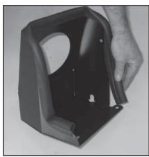
15. Install the provided edge trim onto the heat shield.
