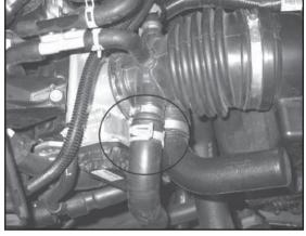
3. On vehicles equipped with an air injection pump, using pliers, release the spring clamp that fastens the air injection hose to the factory intake tube, then disconnect the air injection hose from the intake tube.
