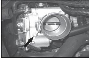
18. Remove the lower throttle body bolt. **Note: Bolt will be Re-used.**
