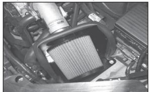
24. Install the K&N air filter onto the intake tube and fasten using the provided hose clamp.
