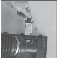
10. Remove the two screws that fasten the mass air sensor to the factory air box, then remove the mass air sensor.
