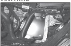
16. Place the heat shield into position in the inner fender well, then fasten using the stock bolts removed in step # 9.
