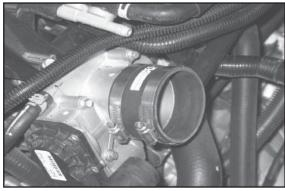
17. Install the provided silicone hose (08440) onto the throttle body and fasten using the provided hose clamp.
