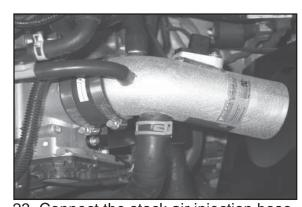
23. Connect the stock air injection hose to the fitting on the K&N intake tube, then fasten using the stock spring clamp.
