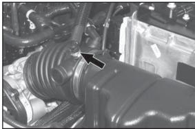
3a. On vehicles equipped with an EVAP vent line, cut the clamp that secures the vent line elbow to the stock intake tube. Then, remove the EVAP vent from the intake tube as shown.
