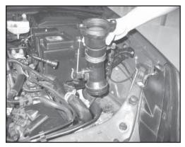
8. Loosen the hose clamp that fastens the mass air sensor housing to the air filter housing, then remove the mass air sensor housing.
