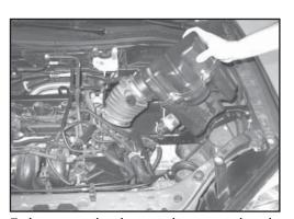
5. Loosen the hose clamp at the throttle body, then lift firmly, separating the upper intake housing from the mass air sensor housing and throttle body. Remove the upper intake housing.
