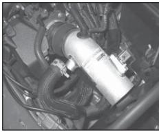
24. Install the K&N intake tube into the silicone hose previously installed onto the throttle body. Align the intake tube with the previously installed intake tube mounting bracket; fasten using the respective hose clamp and hardware.
