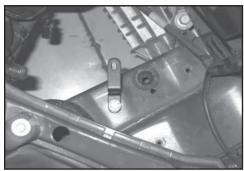
17. Install the heat shield mounting bracket (06488) onto the inner fender; fasten using the provided hardware.
