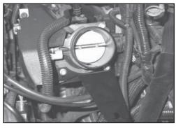
13. Install the intake tube mounting bracket onto the throttle body, then fasten using the throttle body bolts removed in step # 12.
