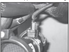
6. Disconnect the mass air sensor electrical connection. Press the locking tab, then gently pull away from the housing.
