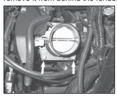
12. Remove the two lower throttle body bolts.
