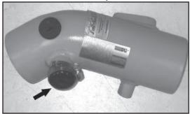
19c. On vehicles not equipped with an air injection pump, install the provided caplug onto the air injection fitting and secure with the provided hose clamp as shown.
