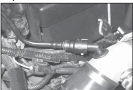
27. Connect the crank case vent hose to the stock fitting previously installed into the K&N intake tube.
