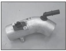
23. Install the provided grommet and stock crank case vent fitting into the K&N intake tube.
