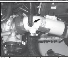
26. Connect the air injection hose to the K&N intake tube and fasten using the stock spring clamp.
