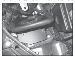
18. Place the heat shield into position onto the inner fender well heat shield mounting bracket and align the second heat shield bracket with the threaded hole in the inner fender. Fasten the heat shield using the provided hardware.
