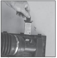
8a. Remove the two screws that fasten the mass air sensor to the factory air box, then remove the mass air sensor.
