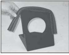
14. Install the edge trim onto the heat shield.
