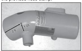
19a. On vehicles equipped with an EVAP vent line, drill a 5/8" I.D. hole in the tube at the location shown.
