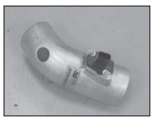
21. Install the mass air sensor into the K&N intake tube, then fasten using the provided hardware.
