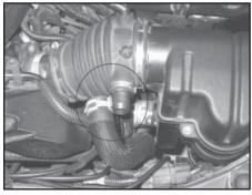
3. On vehicles equipped with an air injection pump; using pliers, release the spring clamp that fastens the air injection hose to the stock intake tube. Disconnect the air injection hose from the stock intake tube.
