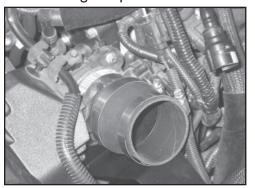
19. Install the silicone hose (084016) onto the throttle body and fasten with the provided hose clamp.
