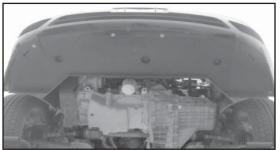
13b. On vehicle's that were equipped with the splash shield, reinstall with the bolts removed in step #8b.
