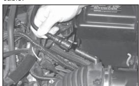
2. Remove the crank case vent hose by pressing the green locking tab and gently pulling the crank case vent hose away from the fitting.
