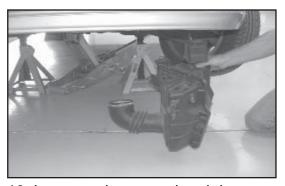
10. Lower and remove the air box assembly from the vehicle.
