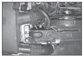
8c. On vehicle's equipped with an air box cover, remove the two bolts which secure the cover to the frame rail, and the bolt which secures the intake snorkel to the radiator core support.
