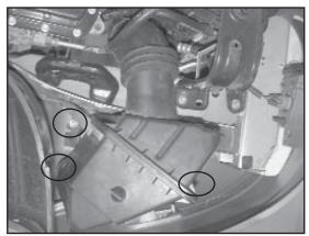
9. Remove the three bolts that fasten the lower air box to the inner fender well.
