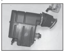
22. Remove the crank case vent fitting from the stock intake tube.
