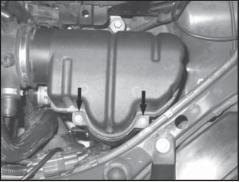
4. Loosen the two bolts that fasten the upper intake housing to the mass air sensor housing.
