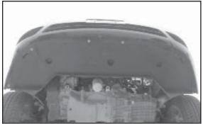
8b. On vehicles equipped with the splash shield, remove the six bolts and five black plastic screws which secure the splash shield to the bumper cover, then remove the splash shield from the vehicle.
