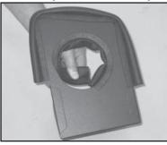
15. Install the edge trim onto the center portion of the heat shield.
