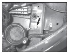
7. Remove the bolt that fastens the mass air sensor housing bracket to the inner fender.
