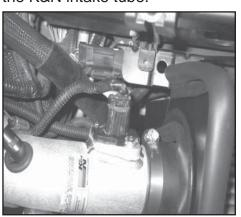
28. Re-connect the mass air sensor electrical connection.
