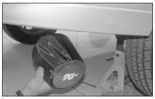
24. From underneath the vehicle, install the K&N Air filter onto the K&N intake tube and tighten hose clamp completely.
