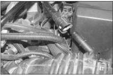
2. Depress the green locking tab on the crank case vent hose and then pull the vent hose to disconnect from the fitting as shown.
