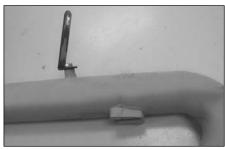
17. Install the supplied "L" bracket and hardware to the K&N intake kit. Do not tighten completely. **NOTE**: Before installing the "L" bracket, inspect the inside of the tube for any debris, then clean the inside out with water and a towel. Inspect the tube one more time before proceeding to the next step.
