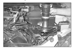
9. Pull firmly up and remove the mass air sensor assembly from the vehicle.
