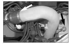
20. Install the K&N intake tube into the vehicle by inserting one end onto the throttle body silicone hose then making sure that the "L" bracket lines up ont the rubber mounted stud.
