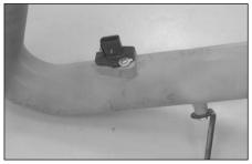
19. Using the stock bolts removed in step # 13, install the mass air sensor into the K&N intake tube as shown.
