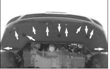
10a. On vehicle's equipped with the splash shield, remove the six bolts and five plastic screws which secure the splash shield to the bumper cover, then remove the splash shield from the vehicle.
