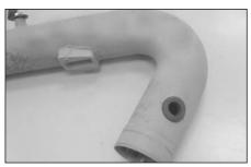
18. Install the supplied rubber grommet into the K&N intake tube as shown.
