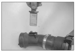
16. Remove the mass air sensor from the stock secondary tube.
