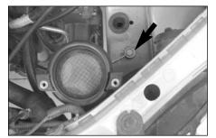
8. Remove the bolt, which secures the mass air sensor housing bracket to the inner fender.
