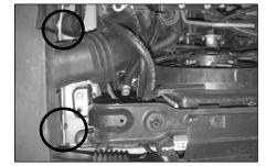
11. On vehicle's equipped with an air box cover, remove the two bolts which secure the cover to the frame rail, and the bolt which secures the intake snorkel to the radiator core support.
