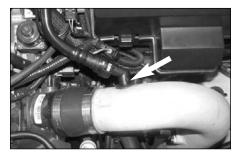
21. Insert the crankase vent line into the rubber grommet on the K&N intake tube as shown.
