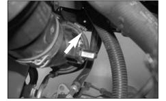
7. Loosen the hose clamp, which secures the mass air sensor housing to the lower intake housing.
