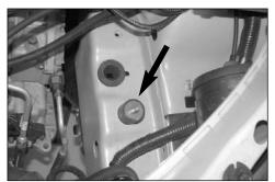
15. Install the supplied rubber mounted stud to the factory threaded hole as shown.
