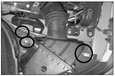
13. Remove the three bolts which secure the lower air box to the inner fender well.
