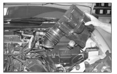
5. Lift firmly to separate the upper intake housing from the mass air sensor housing and then remove the upper intake housing from the vehicle.
