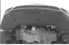
26. On vehicle's that were equipped with the splash shield, reinstall with the bolts removed in step #10a.
