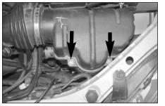
4. Loosen the two bolts, which secure the upper intake housing to the mass air sensor housing. **NOTE:** The two bolts do not separate from the upper intake housing.
