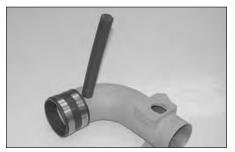
17. Install the provided silicone hose onto the vent on the K&N Typhoon intake tube as shown.
