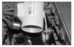
20. Line up the tube bracket with the rubber mounted stud and secure with the provided hardware as shown.
