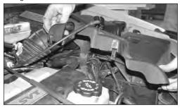
4. Pull up firmly to remove the plastic coil cover as shown.
