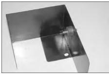
11. Install the rubber mounted stud onto the heat shield and secure it with the provided hardware as shown.
