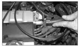
5. Disconnect the crank case vent hose from the cam cover as shown.
