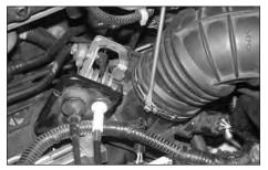
6. Remove the clamp at the throttle body as shown.
