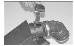
15. Remove the mass air sensor from the stock air cleaner assembly as shown using the provided Torx wrench.
