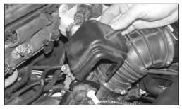
3. Pull up firmly to remove the plastic throttle linkage cover as shown
