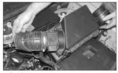
7. Pull firmly upwards to remove the air cleaner assembly as shown.
