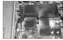
12. Install the heat shield into the vehicle and slide the slot on the heat shield onto the bolt from step 9, then, line up the hole with the rubber mounted stud from step 10 as shown.
