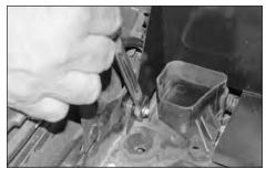
14. Tighten the hex nut on the heat shield as shown.
