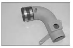
16. Install the silicone hose and hose clamps onto the K&N Typhoon intake tube as shown.
