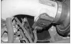
24. Reconnect the mass air sensor electrical connection as shown.
