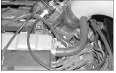
23. Reconnect the crank case vent hose to the cam cover as shown.
