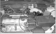
27. Reconnect the negative battery cable and double check to make sure everything is tightened and properly positioned before starting the vehicle.
