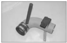
18. Install the mass air sensor into the tube and secure with the provided hardware as shown.
