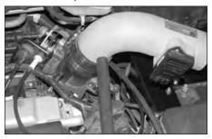
19. Install the tube into the vehicle and onto the throttle body as shown.
