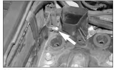
9.Install the provided nut and washer onto the stock bolt on the air cleaner tray as shown.
