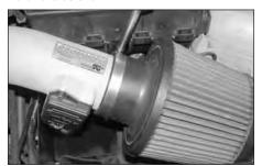
21. Install the air filter onto the Typhoon intake tube and tighten as shown.
