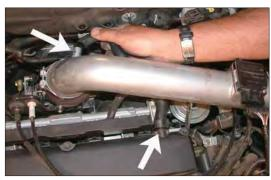
12. Using the provided vent hose, (Trim to fit), connect to the K&N Typhoon intake tube and valve cover as shown.
