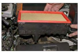
6. Pull firmly upwards to remove the lower air cleaner assembly as shown.
