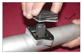
9. Install the mass air sensor into the K&N Typhoon intake tube using the stock bolts from step 8.
