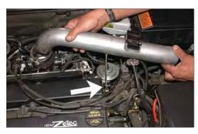
11. Install the K&N Typhoon intake tube into the silicone hose then line up the bracket with the ignition bracket and secure with the bolt from step 10. Tighten the hose clamps using the 9/64 allen wrench provided.
