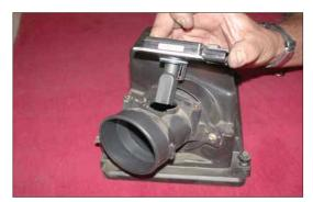
8. Remove the two bolts that secure the mass air sensor, then, remove the mass air sensor as shown.
