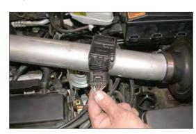
14. Reconnect the mass air sensor electrical connection as shown.
