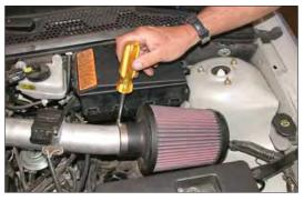
13. Install the K&N air filter onto the K&N Typhoon intake tube and tighten with the provided hose clamp as shown.
