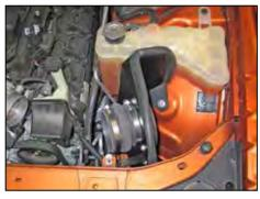
13. Set the heat shield assembly into position in the engine bay so the rubber insert passes into the air box mounting hole in the inner fender. Do not secure the heat shield at this time.
