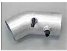
17. Install the inlet air temperature sensor into the K&N® intake tube as shown.
