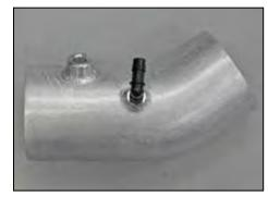
15. Install the provided 90° vent fitting into the  $K\&N^{\otimes}$  intake tube as shown.
