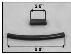
19. Cut the provided ½" silicone vent hose to a length of 9" long. Also cut the 5/8" vent line to a length of 2.5" long.
