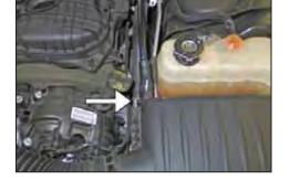
4. Disconnect the crankcase vent hose from the air filter housing.
