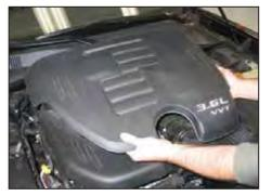
2. Lift up and remove the engine cover and remove it from the engine.
