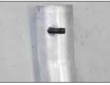
18. Install the 90° NPT fitting into the K&N $^{\mbox{\tiny \$}}$  intake tube as shown.
