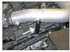
22. Install the tube bracket onto the mounting stud and then secure to the K&N<sup>®</sup> intake tube with the provided hardware. Tighten the hose clamps at this time.
