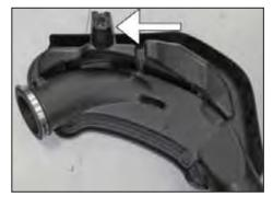
20. Remove the intake plenum mount grommet from the intake plenum.
