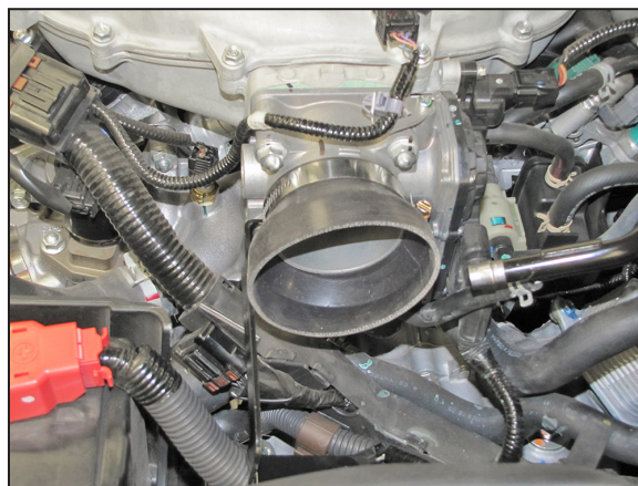
16. Install the provided silicone hose (084093) onto the throttle body and secure with the provided hose clamp. NOTE: The hose is a tight fit onto the throttle body.
