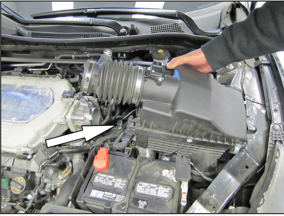
7. Lift up the air box half way out, then unhook the wiring harness from the air box and remove the air box assembly.
