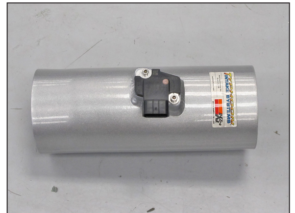
18. Install the mass air sensor into the K&N® intake tube and secure with the provided hardware.
