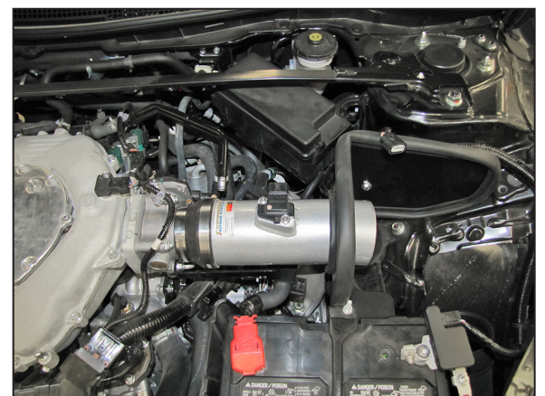
20. Install the K&N® intake tube through the heat shield and then into the silicone hose, and then align with the mounting bracket. Secure the tube with the provided hose clamp and hardware.
