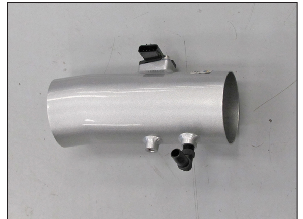
19. Install the 90° vent fitting into the K&N® intake tube as shown. NOTE: Plastic NPT fittings are easy to cross thread. Install the vent fitting "hand" tight, then turn it two complete turns with a wrench.
